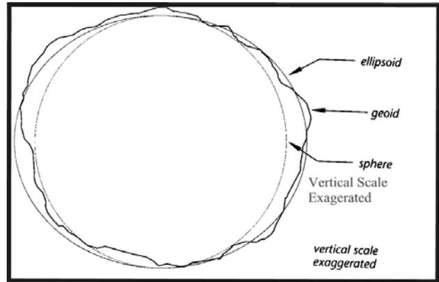
Figure 21: Earth's Surface and its Modeling
