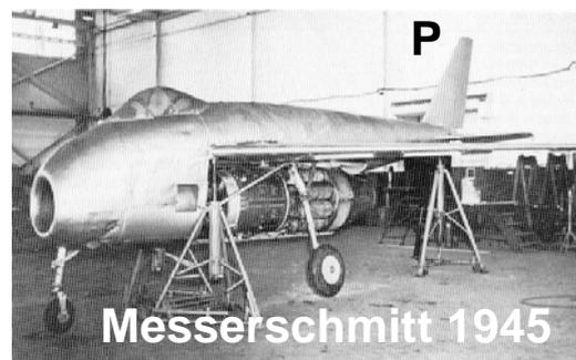
Figure 8: Swept wing aircraft for high subsonic speed reduced compressibility effects
