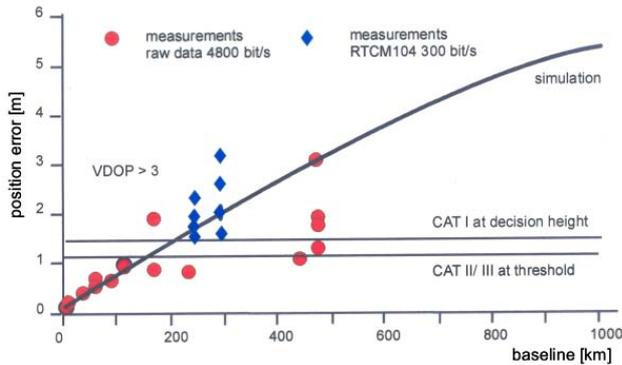
Figure 20: DGPS vertical accuracy
