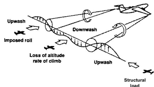
Figure 56: Response of aircraft when passing a wake vortex
