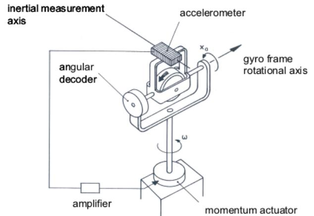
Figure 12: Basic principle of inertial navigation (single axis)
