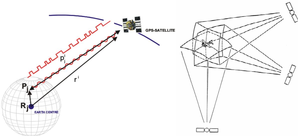
Figure 16: Basic principle of satellite navigation
