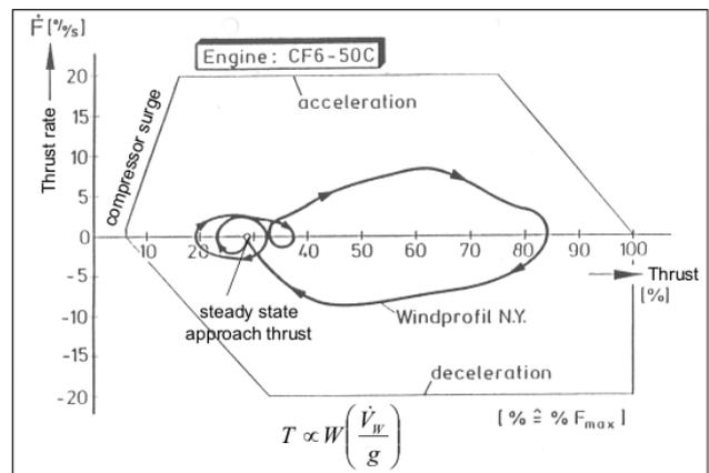
Figure 51: Phase diagram of required thrust in a simulated thunderstorm accident (B727, New York 1975)
