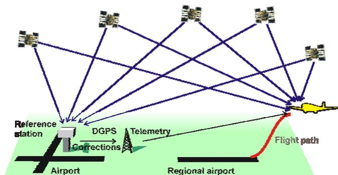
Figure 19: Differential satellite navigation principle
