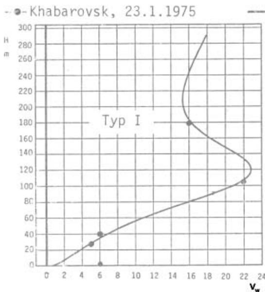
Figure 52: Strong wind shear in Khabarovsk (1975) causing a Fatal Accident
