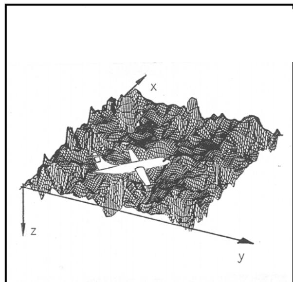
Figure 41: Airplane passing a two-dimensional turbulence field
