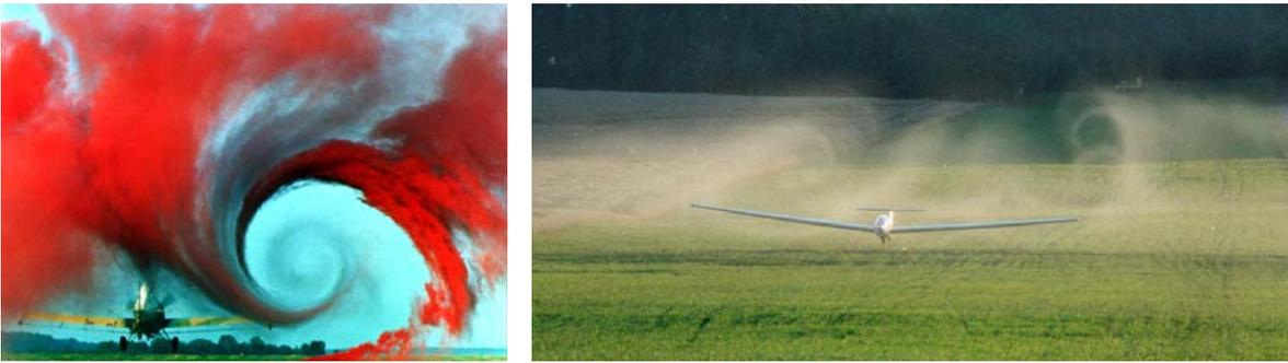
Figure 39: Wake vortices behind aircrafts
