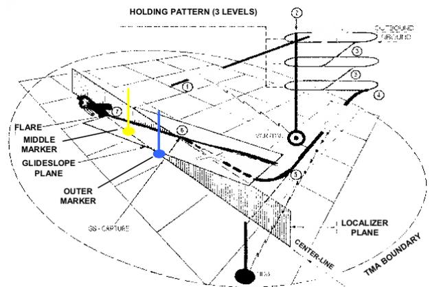
Figure 7: Instrument landing system
