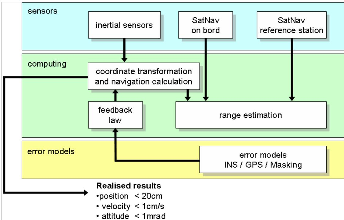
Figure 22: Integrated navigation system
