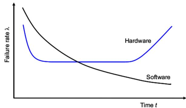
Figure 38: Typical failure rates of control systems hardware and software
