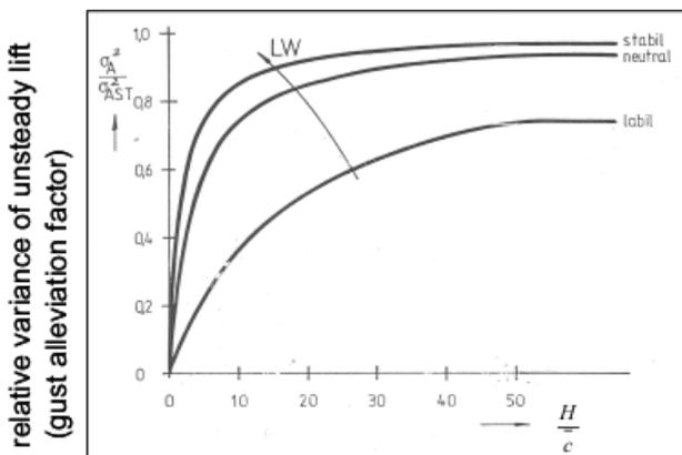
Figure 48: Gust alleviation factor as a function of relative height above ground
