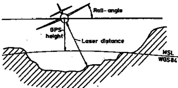
Figure 26: Contour measurement of mountainous regions (principle)
