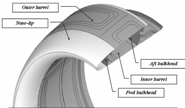
Figure 1. Turbofan intake structural scheme.
