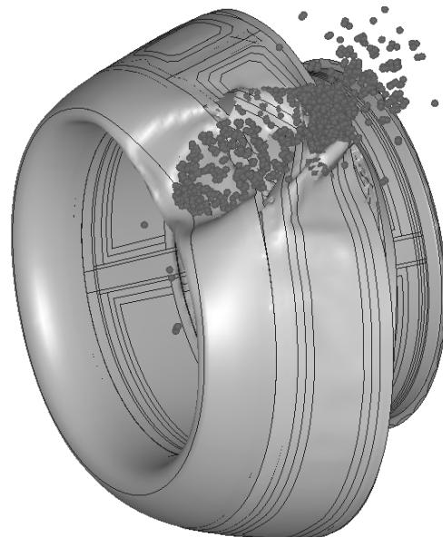
Figure 4. Birdstrike onto a turbofan-engine intake.
