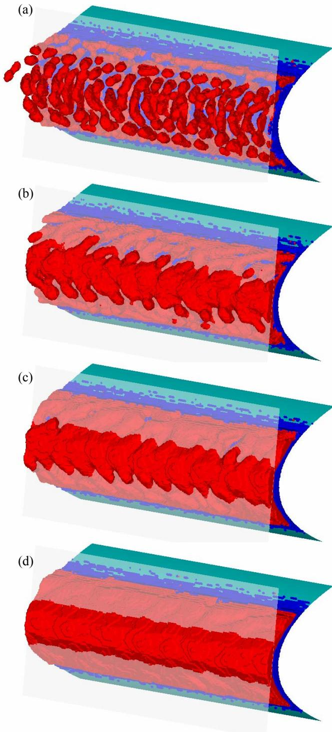
Fig. 6. Predicted lobster tail (scallop) ice shapes forming on a swept wing with a sweep angle of  $30^\circ$  and varying freezing range parameter.
