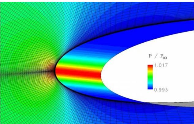
Fig. 4. Predicted flow field for a sweep angle of  $45^\circ$ . The computational grid used for the simulation is also shown.
