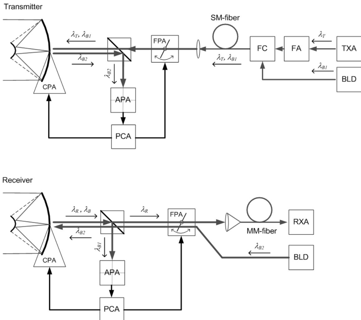
Fig. 8 Basic terminal concept for a simplex link; PAT based on beacon approach: The beacon-wavelength is separated in the receiver from the data-wavelength using a chromatic beam splitter.
