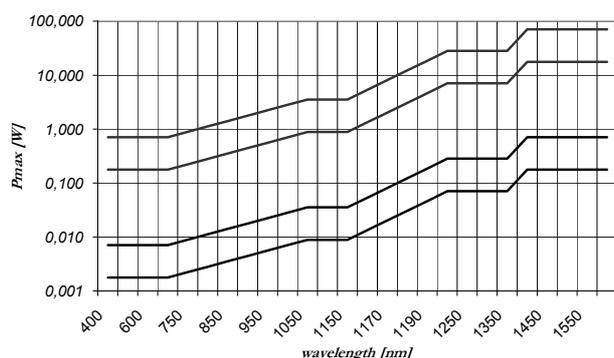
**Fig. 4** Maximum terminal transmit power  $P_{max}$  [W] for cornea exposure vs. wavelength [nm] for the FWHM-divergence angles  $50$  (lowest curve),  $100$ ,  $500$  and  $1000 \mu rad$  (uppermost curve) and a distance to the transmitter of  $300$  m (minimum in-flight A/C distance due to air-traffic regulations)
