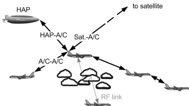
**Fig. 1 Application scenarios for aeronautical optical links**
