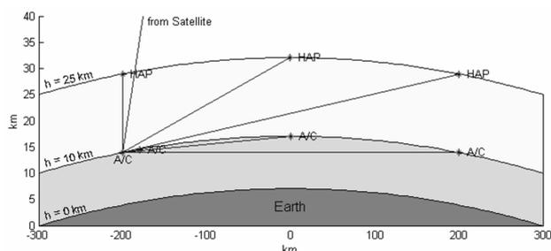
**Fig. 2 FSO link distances for links between A/C, HAP and satellites**
