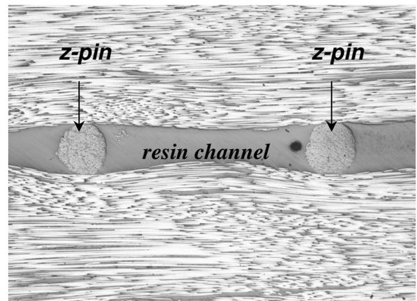
Fig. 2. Continuous resin channel along a row of z-pins.
