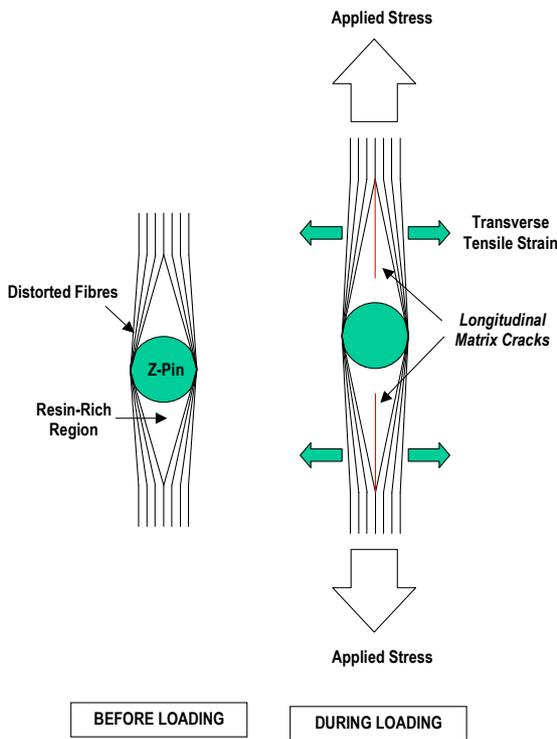
Fig. 6. Schematic of the failure mechanism that causes longitudinal splitting of the z-pinned composites under monotonic tensile loading.
