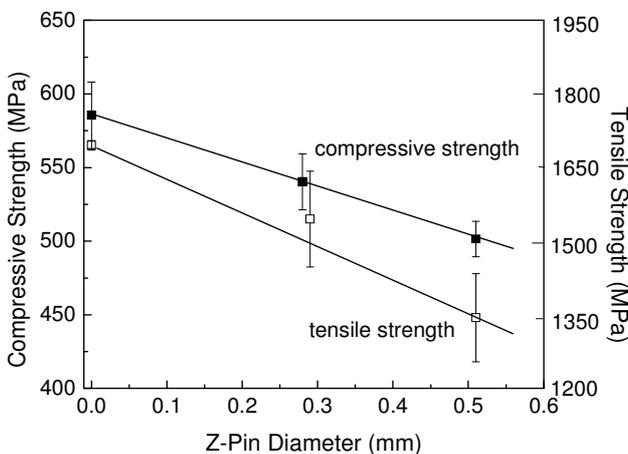
Fig. 4. Effect of z-pin diameter of the tensile and compressive strengths.
