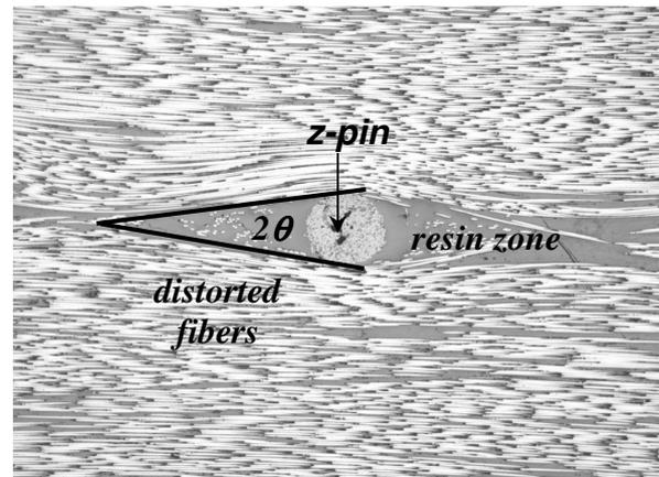
Fig. 1. Local fiber distortion and resin-rich zones surrounding a z-pin.
