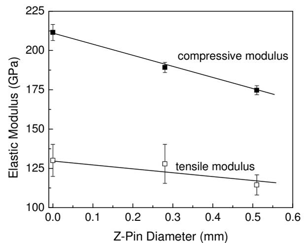
Fig. 3. Effect of z-pin diameter of the tensile and compressive moduli.
