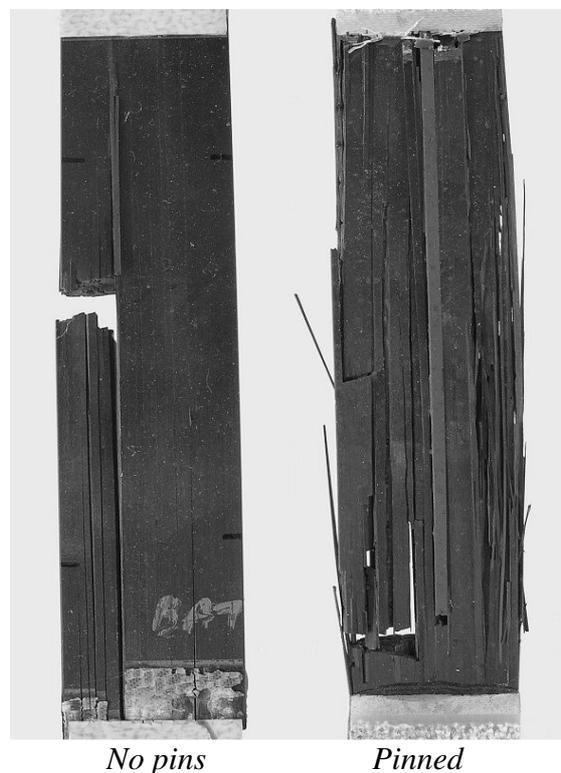
Fig. 5. Photographs of unpinned and z-pinned composite specimens broken under tensile loading.
