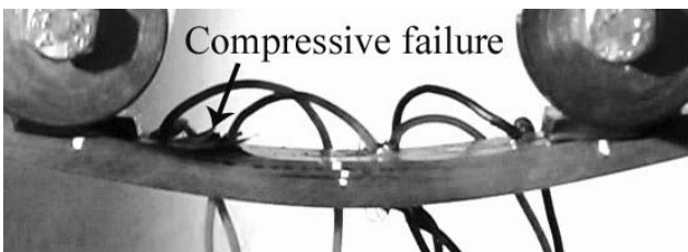
Fig. 5. Failure mode in the reference test
