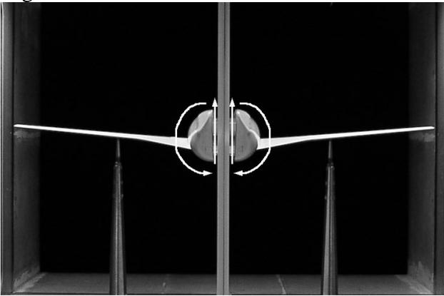
Fig. 11: Additional circulation around the fuselage
