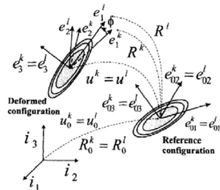
Fig. 10 Revolute joint in the reference and deformed configurations. {cf. [4]}
