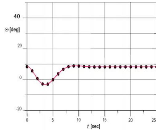
Fig. 17 Results of simulations. Course of pitch angle - no friction and free-play in control system
