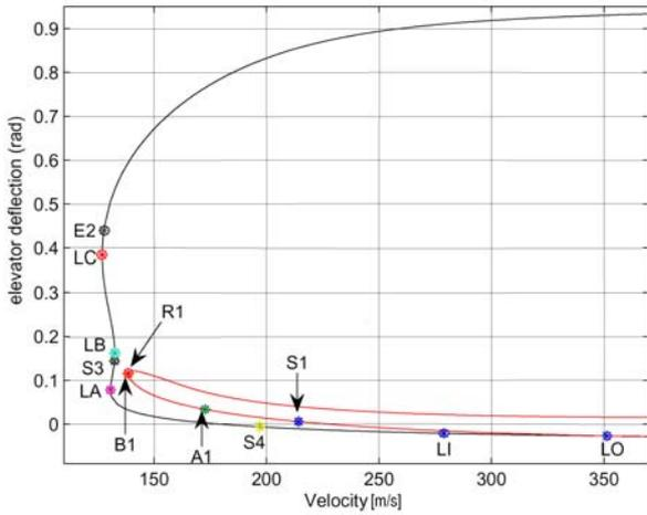
Fig. 13 Bifurcation curves of the nominal and reconfigured systems with single actuator failures and velocity as the parameter
