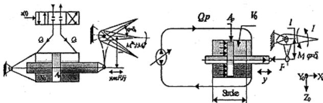
Fig. 1 The simplified model of the elevator's hydraulic servo-actuator
