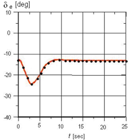
Fig. 16 Results of simulations. Deflection of elevator - no friction and free-play in control system
