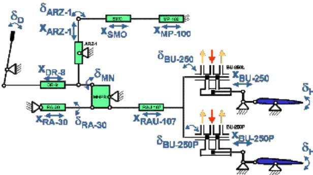
Fig. 4 The kinematic scheme of the Su 22 fighter aircraft longitudinal control system
