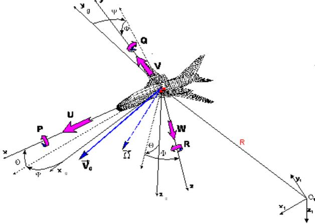
Fig. 3 System of co-ordinates attached to the aircraft
