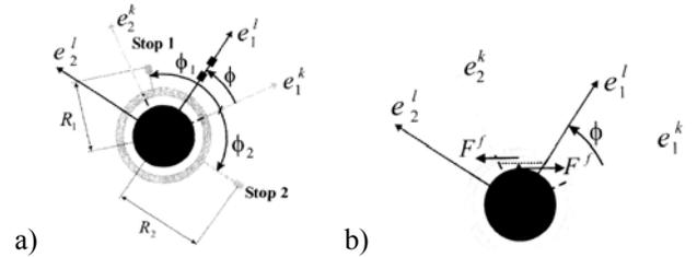
Fig. 11 a) A revolute joint with backlash. The magnitude of the relative rotation  $\phi$  is limited by the stops; b) A revolute joint with friction. (cf. [4])
