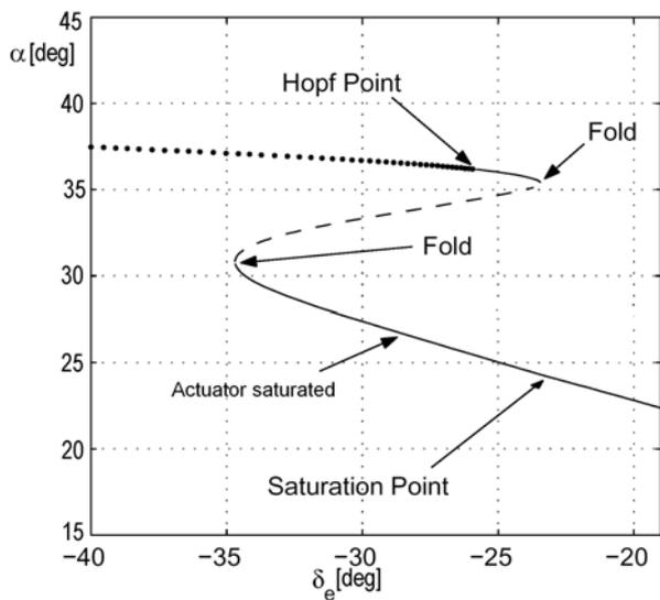
Fig. 15 Bifurcation curve of the system with actuator saturation – high  $\alpha$  branch
