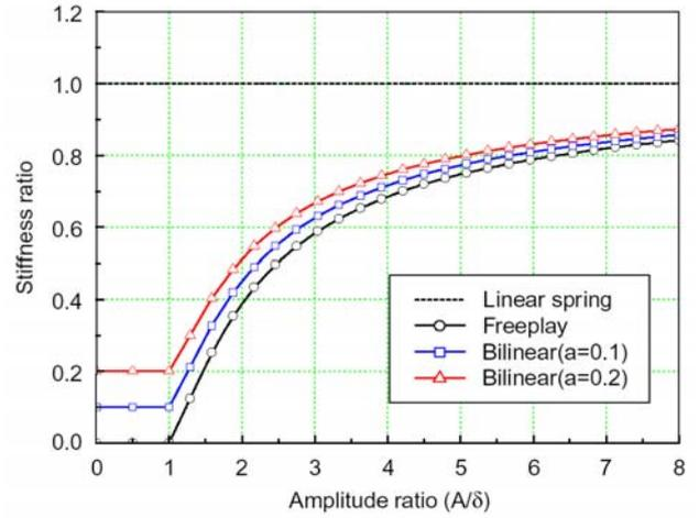
Fig. 6 Equivalent stiffness of nonlinear spring.
