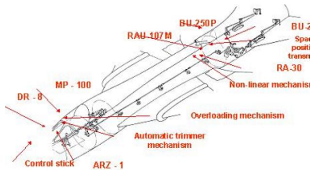
Fig. 2 Scheme of the Su-22M fighter aircraft longitudinal control system
