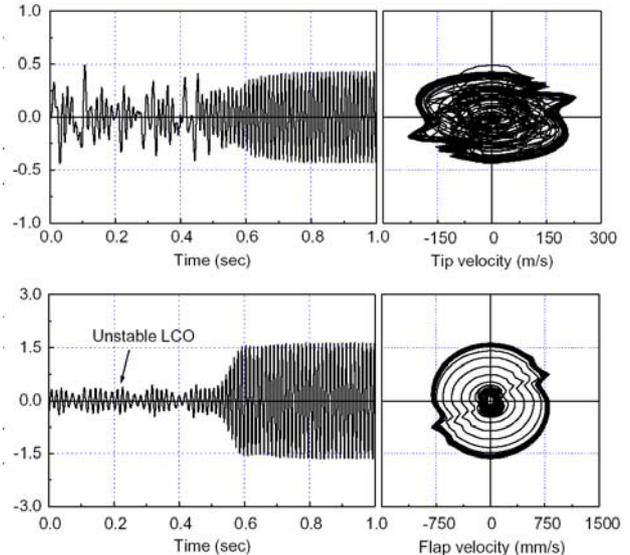
Fig. 8 Example of simulation of elevator motion ( $\theta/\delta=1.0$ )
