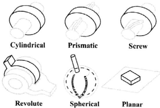
Fig. 9 The six lower pairs.
