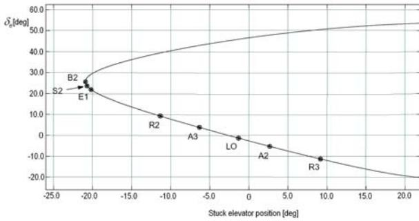
Fig. 14 Bifurcation curve of the system with a stuck elevator and the stuck position as the parameter.
