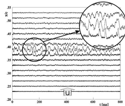
**Fig. 13** Time traces of the PVDF sensors on the A320 HLF Fin
