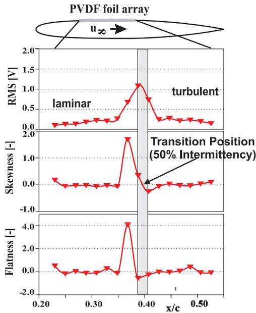
**Fig. 14** Transition detection on the fin with RMS-values, skewness and flatness
