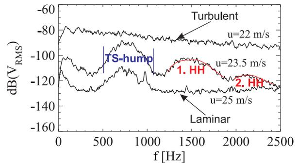
**Fig. 10** Frequency spectra of a surface hot-wire sensor at a 50% chord length at three different flight velocities
