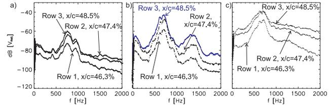
**Fig. 12** Spectra of one microphone sensor per row at three flight velocities, a)  $25\text{m/s}$ , b)  $23.6\text{m/s}$  and c)  $22.2\text{m/s}$
