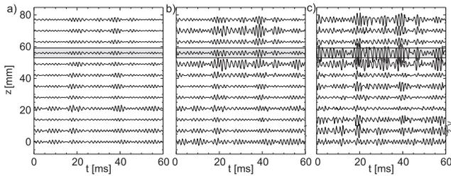
**Fig. 11** Filtered time traces of microphone sensors at a velocity of  $23.6\text{m/s}$  a) row1,  $x/c = 46.3\%$ , b) row2,  $x/c = 47.4\%$ , c) row3,  $x/c = 48.5\%$
