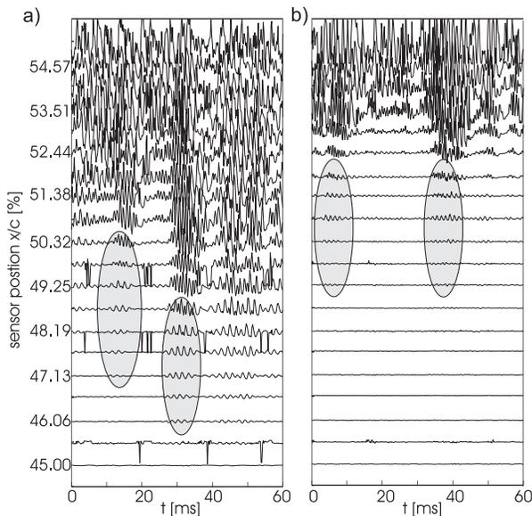
**Fig. 9** Raw signals of the streamwise arranged surface hot-wire sensors a)  $u_\infty = 22.2\text{ m/s}$  and b)  $u_\infty = 27.8\text{ m/s}$
