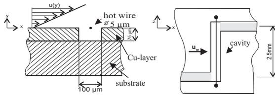
**Fig. 5** Sketch of a single surface hot-wire sensor [1]
