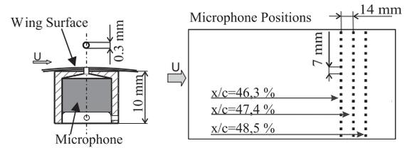
**Fig. 6** Sketch of installation and positions of the miniature microphones
