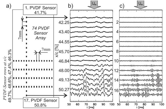
Fig. 8 a) PVDF sensor array, b) raw and c) filtered signals of the streamwise PVDF sensor line at  $u_\infty = 23.6\text{ m/s}$
