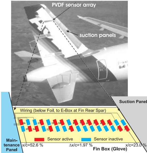
Fig. 3 A320 HLF Fin and the PVDF sensor array
