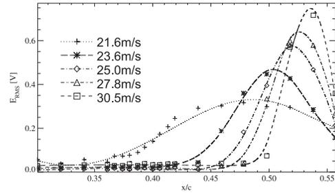
Fig. 7 RMS-values of the streamwise PVDF sensors on the wing glove [9]
