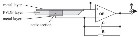
Fig. 4 Sketch of a single PVDF sensor
