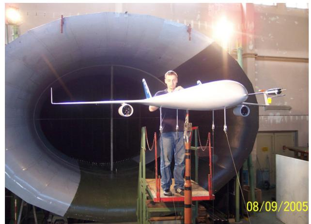
Fig. 3. AC20.30 being mounted in the wind tunnel Dresden-Klotzsche
