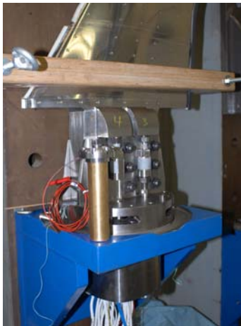
Fig. 11: Wing model assembly during mounting for dynamic qualification in the laboratory; in the foreground one of the four excitation piezo stacks
