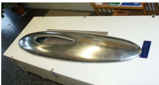
Fig. 7: Fuselage substitute, flow side, labyrinth seal provided around the opening for the wing
