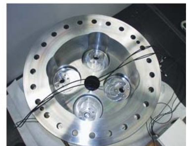
Fig. 13: Inside view of the piezo-6 components windtunnel balance
