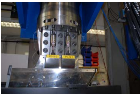
Fig. 12: Wing model with excitation mechanism in the dynamics laboratory
