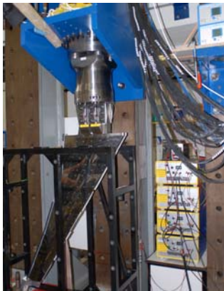
Fig. 22: Cuboidal frame for defining the virtual position reference system
