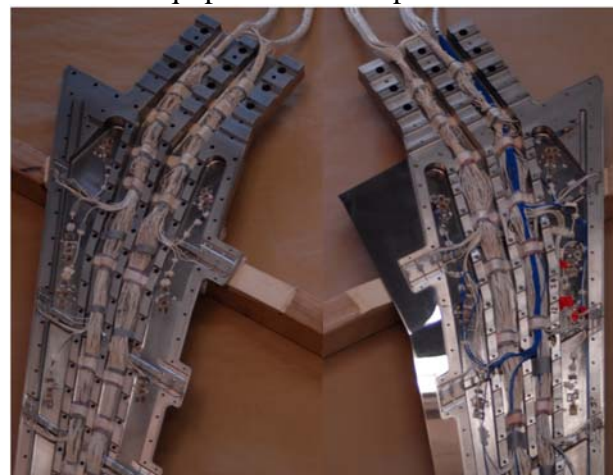
Fig. 17: Sensor installation inside the suction and pressure side parts of the model. Wiring colors: thick white belong to pressure sensors, thin white to strain gauges, blue to accelerometers.
