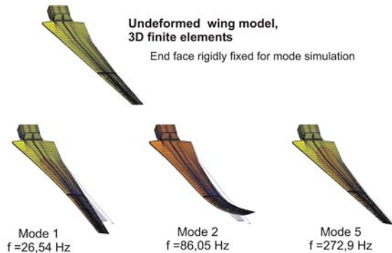
Fig. 10: Two first bending and first torsion mode shapes and eigenfrequencies
