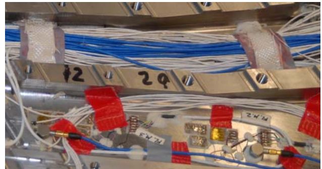
Fig. 20: Close view of sensor application in the suction side part, showing accelerometer and strain gauge applications
