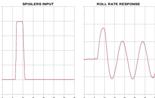
**Fig. 4** Dutch Roll flight test through a spoilers pulse input.
