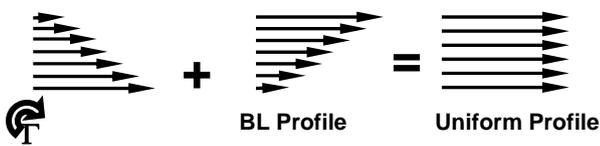
Fig. 2: Velocity Profile Manipulation
