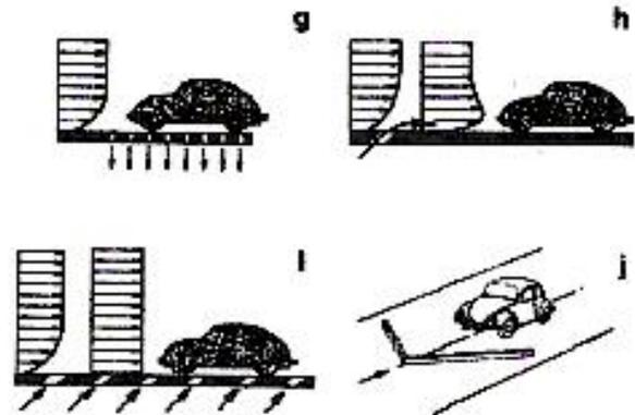
Fig. 1: Boundary Layer Control Techniques [3]
