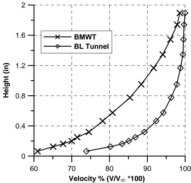
Fig. 9: Boundary Layer Profile Comparison
