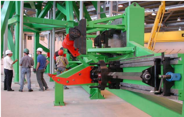
Fig. 8 Iron Bird air load simulation
