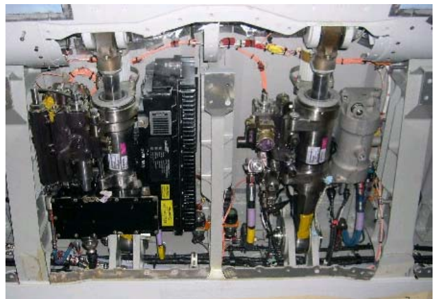
Fig. 5 Aileron EHA and hydraulic actuator
