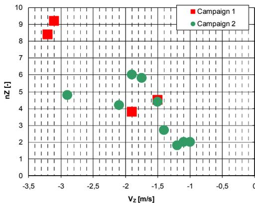
Fig. 3 – Load factors at touch down
