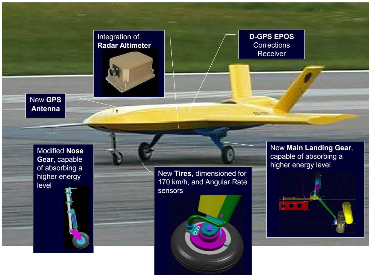
Fig. 4 – Modifications on the platform introduced for the ATOL effort
