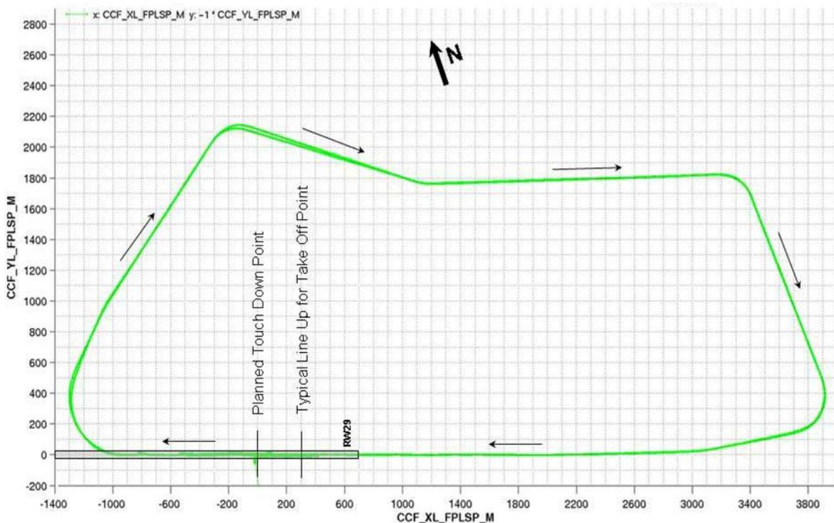
Fig. 6 - Ground track recorded during a mission that was run twice, showing the almost perfect overlay of the flight paths (longitude and latitude in meters on the X- and Y- axis)
