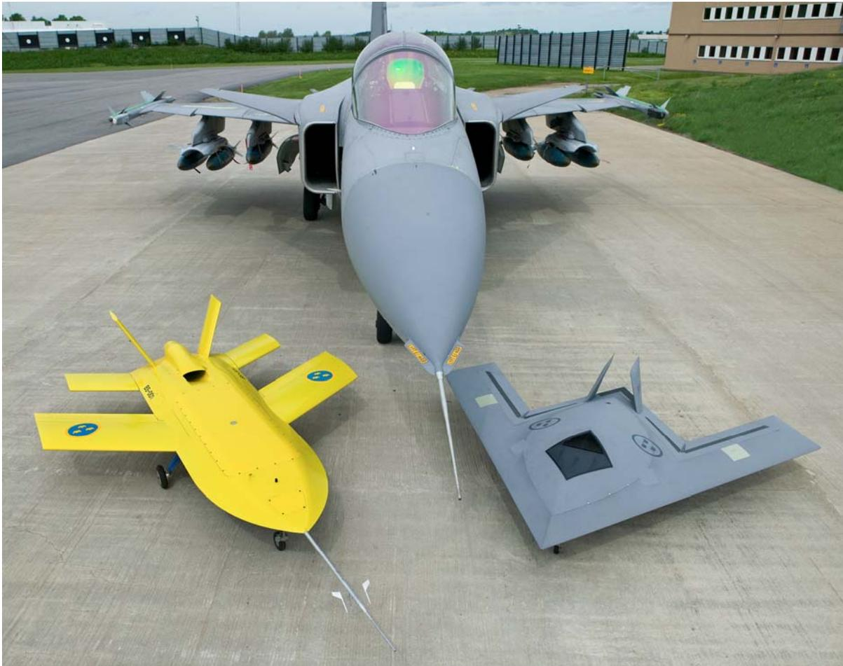
Fig. 0 – SHARC (left) and FILUR (right) with a *JAS39 Gripen* on the background
