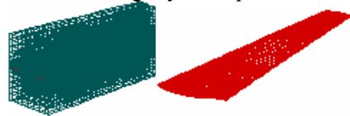
**Fig. 13 Field-Panel Model and CFL3D Surface Mesh of a LANN Wing**
