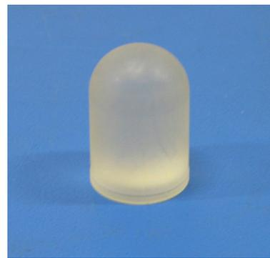
Fig. 6. Spherically Blunted Cylinder Projectile
