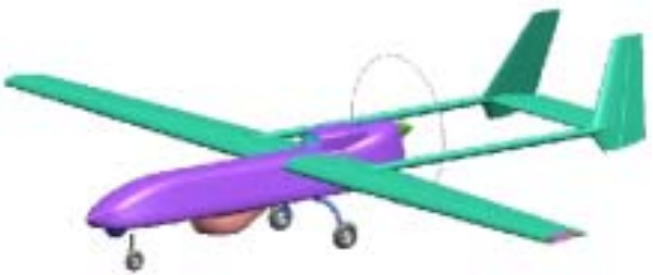
Fig. 21. Tactical UAV powered by fuel cell
