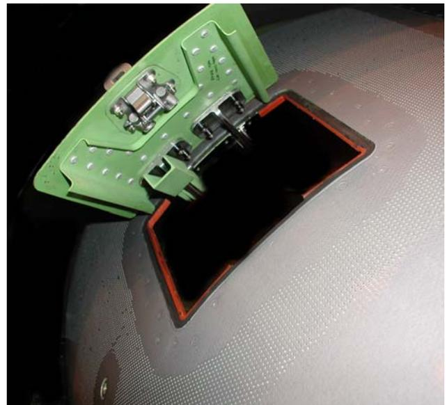
Fig. 1 A typical pressure relief door
