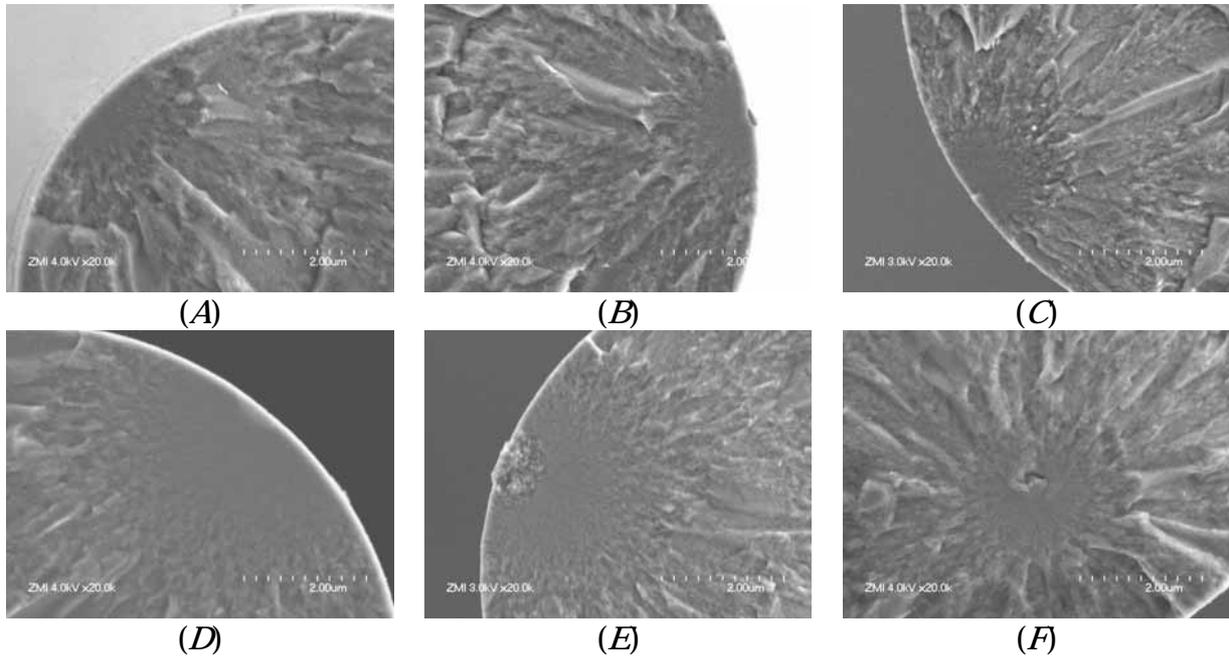
Fig.5 SEM micrographs of each factor group (Example) (A)no trace (B)particle on side face (C)particle in cross-sectional surface (D)crack at side face (E)unhomogeneous structure (F)internal starting point
