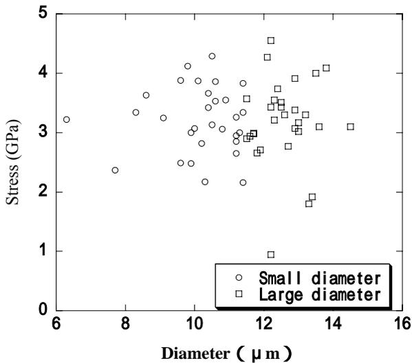
Fig.3 Single fiber tensile test results
