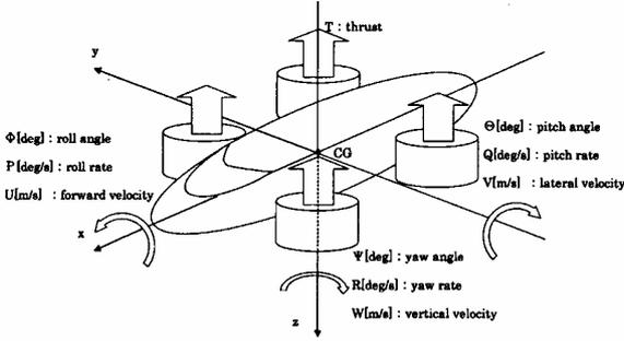
Fig. 1. Body Axes of L/CFA
