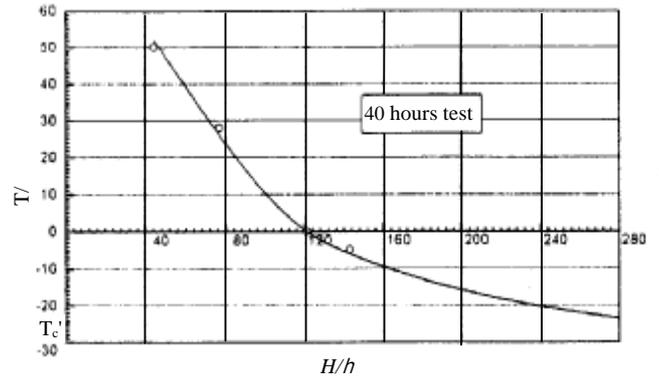
Fig. 2 T-H test curve of average corrosion up to 1 mm for Lc4cs aluminum alloy sheet
