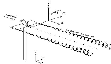
Figure 1 Wing model and coordinate system
