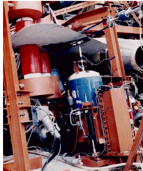
Fig. 10. Rolling Sleeve Airbags (Red) and Electromagnetic Shaker (Blue) in Place on the Horizontal Tail
