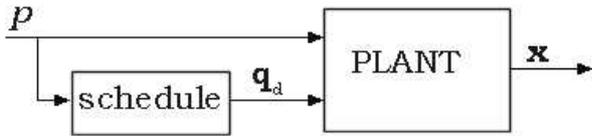
**Fig. 1** Block diagram for the scheduled feedforward control system ("open loop" bifurcation tailoring)
