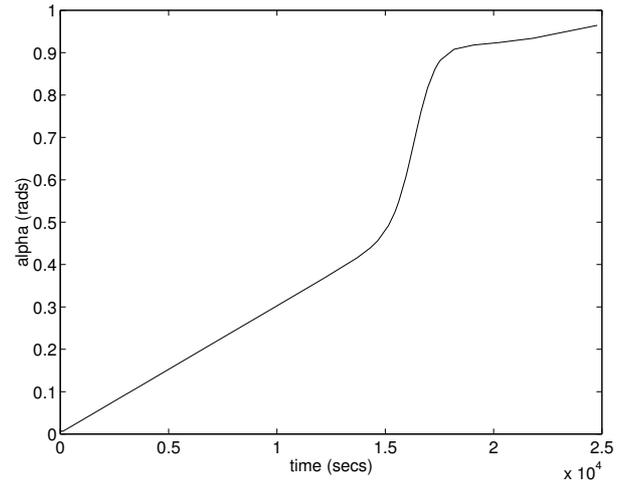
**Fig. 16** Simulation of the HHIRM (including variations from the nominal model) with feedforward scheduling and MCS feedback stabilisation.  $\delta_{el} = -0.001^\circ/s$
