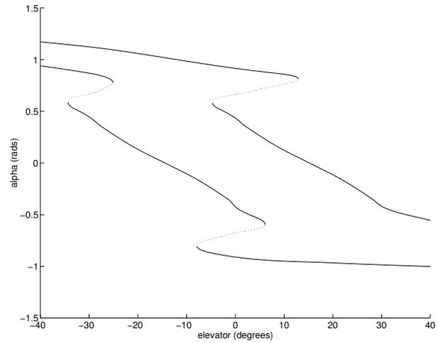
**Fig. 5** Bifurcation diagrams plotted at the limits of  $\delta_{tp}$ . Solid lines = stable, dotted lines = unstable
