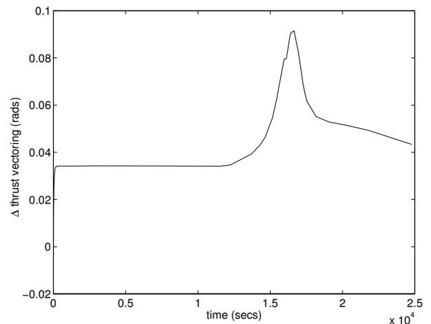
**Fig. 17** Simulation of the HHIRM (including variations from the nominal model) with feedforward scheduling and MCS feedback stabilisation.  $\delta_{el} = -0.001^\circ/s$
