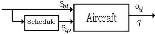
**Fig. 3** Block diagram for the feedforward scheduled (only) HHIRM model
