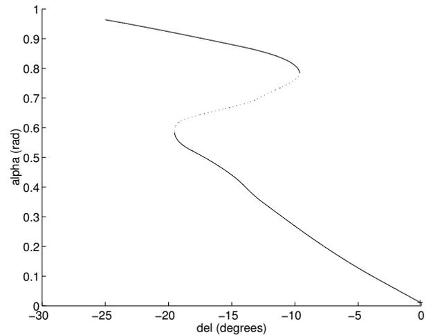
**Fig. 6** Bifurcation plot for the 2nd order HHIRM model with  $\delta_{tp} = 0$  (created using AUTO). Solid lines=stable, dotted lines=unstable.
