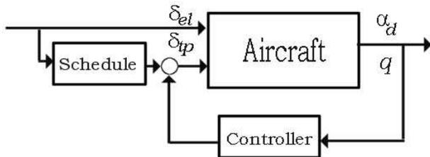
**Fig. 12** Block diagram showing the feedforward scheduled HHIRM model plus feedback stabilisation
