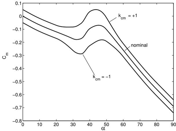
**Fig. 15** The variation in  $C_m$ , the pitching moment coefficient, due to variations in  $k_{cm}$ , the pitching moment coefficient tolerance.
