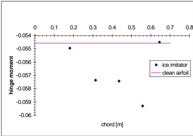
**Fig. 3. Most critical position according to aileron hinge moment**
