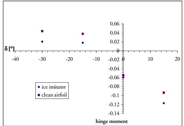
**Fig. 4. Change of hinge moments on the aileron with and without ice imitation according the aileron deflection**
