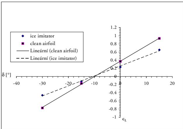
**Fig. 5. Difference in lift coefficients resulting in roll behaviour change**
