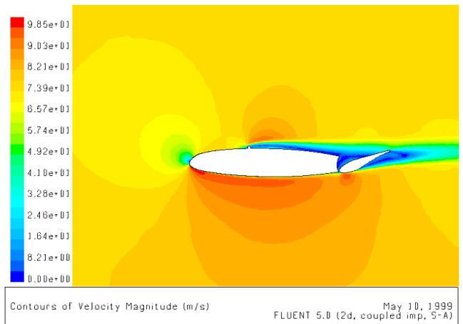
**Fig. 6. The flow field change above the upper surface of the airfoil due to negative aileron deflection**
