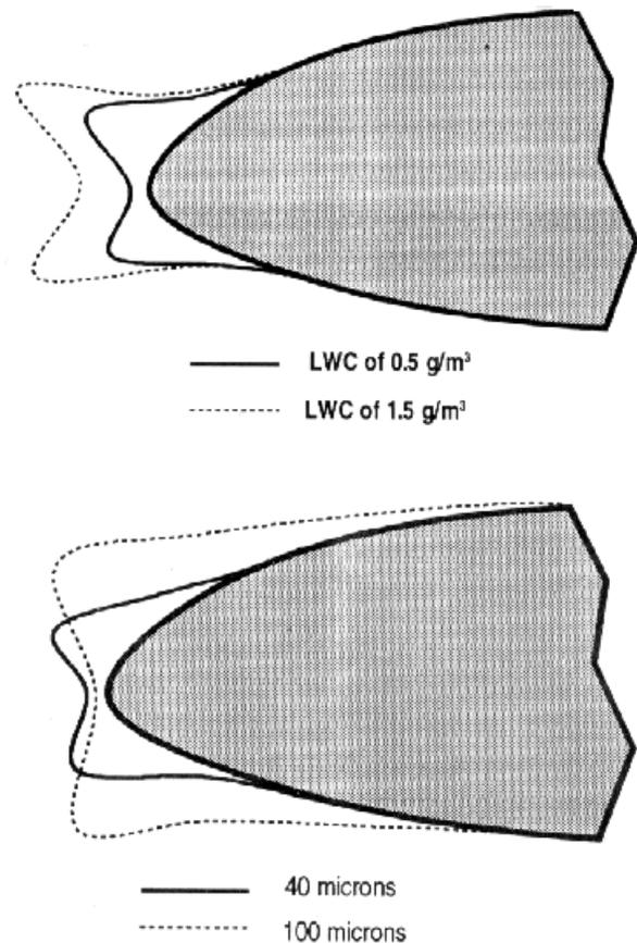
**Fig. 1. Exceedence of condition in FAR 25 – first picture and LWC and MVD influence on ice-accretion position – next two pictures.**
