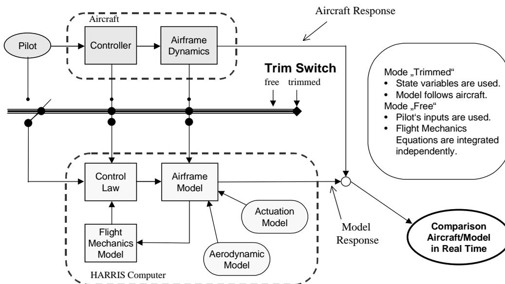
Fig. 3: Flight Mechanic Coupling of On-line Simulation with Telemetry Data
