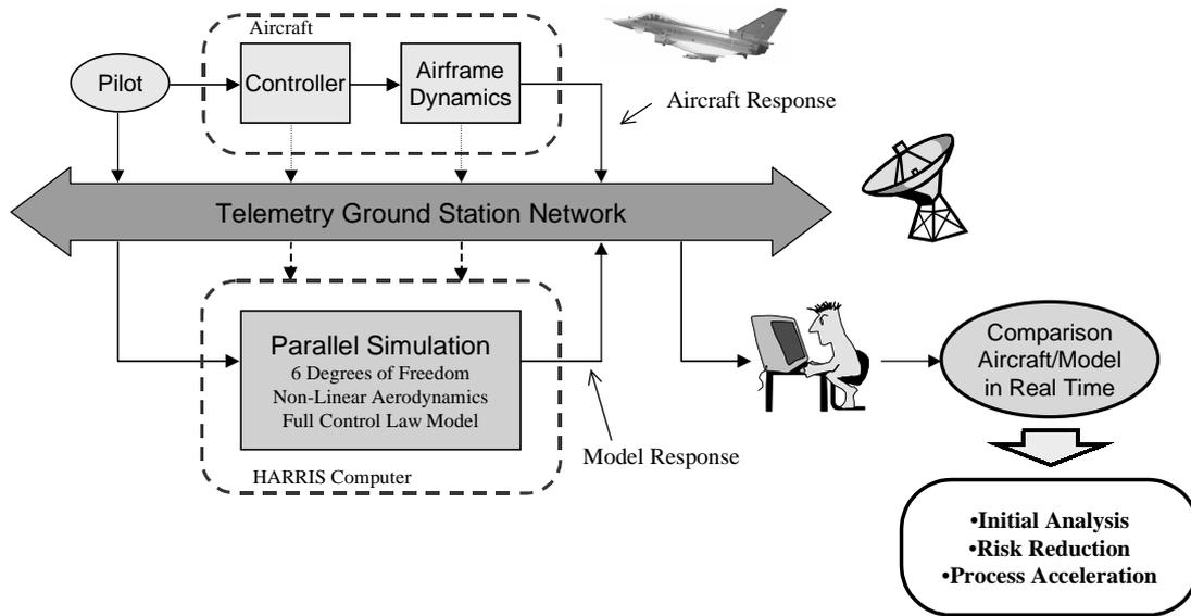
**Fig. 2: Integration of On-line Simulation into Telemetry Network**
