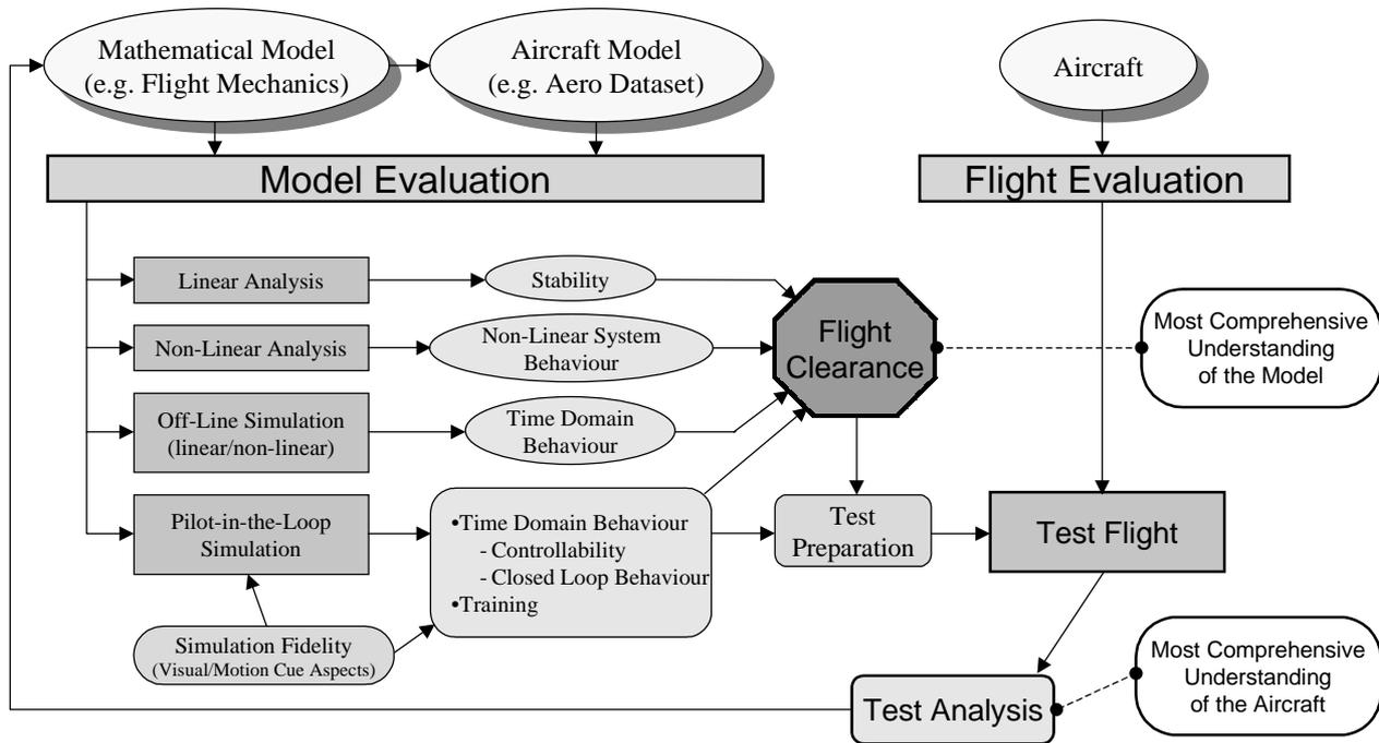
Fig. 1: Simulation and Flight Test
