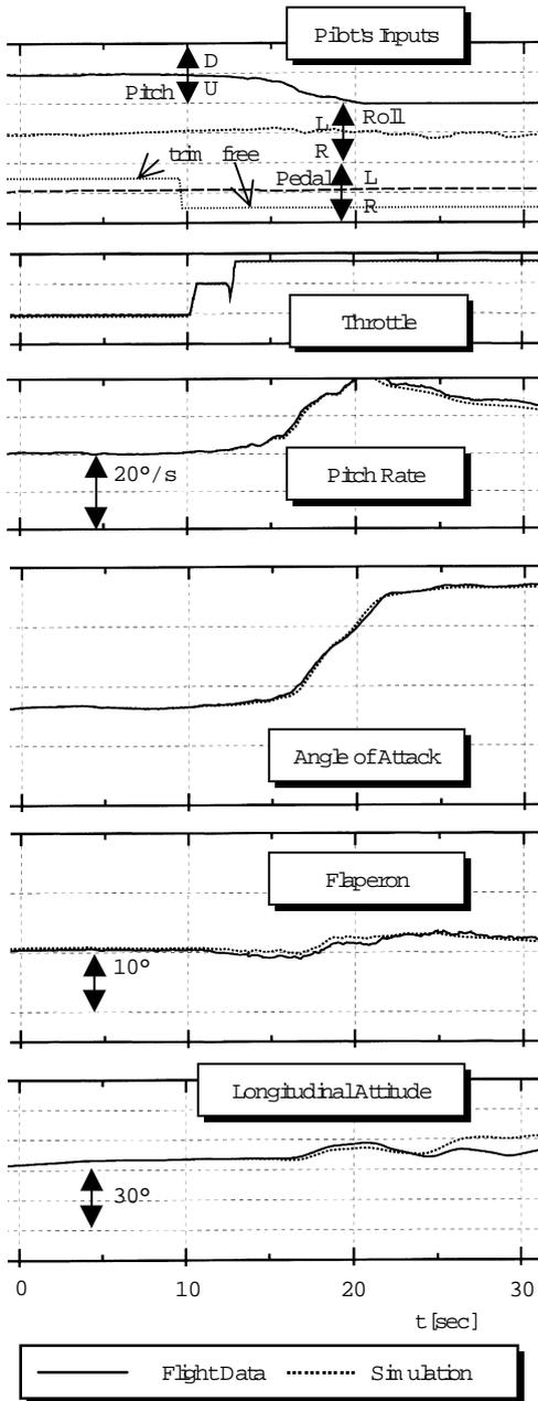
**Fig. 5: On-line Simulation Results for a Wind-up Turn**
