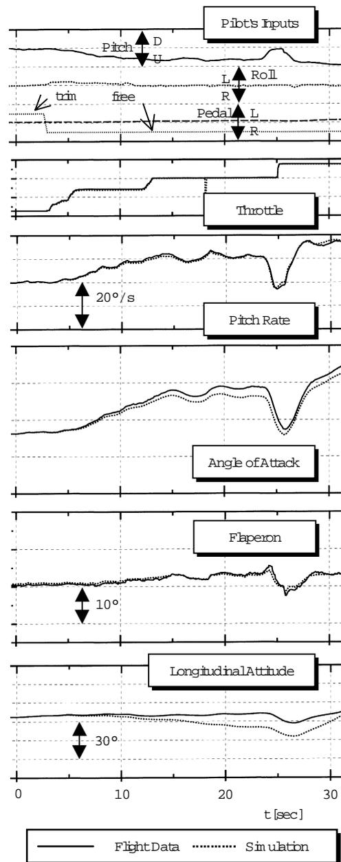
**Fig. 6: On-line Simulation Results for a Turn Manoeuvre**
