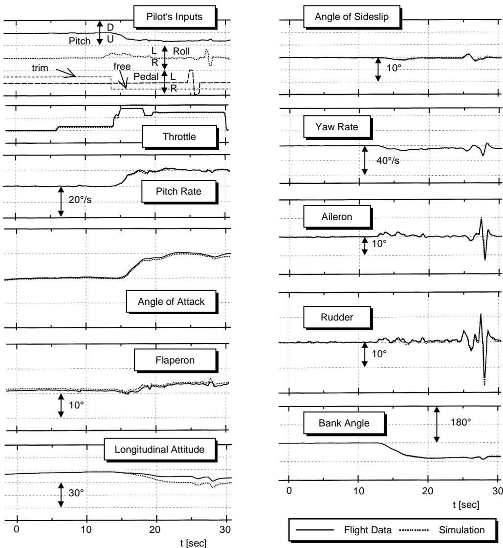
**Fig. 4: On-line Simulation Results for a Yaw-Roll Doublet**
