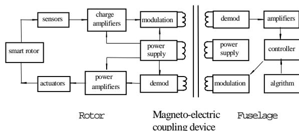
Fig.3 Schematic diagram of non-contact signal transmission system
