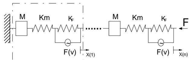
**Fig.2 Mechanical model of the stack actuator**
