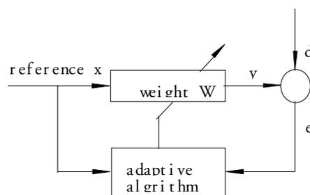
Fig.4 Structure of adaptive filter
