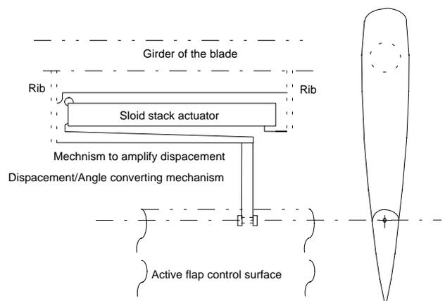
**Fig. 6 Structure of the active flap**
