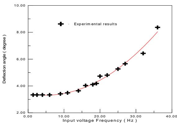
**Fig. 8 Frequency response of the AFC model**
