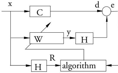
**Fig.5 An adaptive filtered feed forward controller**
