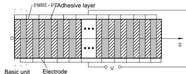
Fig.1 structure of stack actuators
