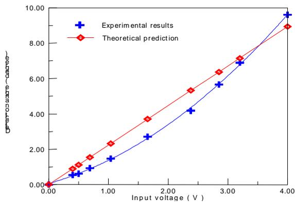
**Fig. 7 Deflection of the AFC in static test**
