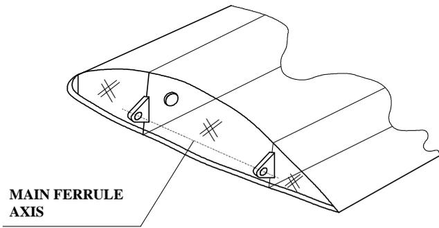
Fig.8. Details of the joining of the main wing to fuselage
