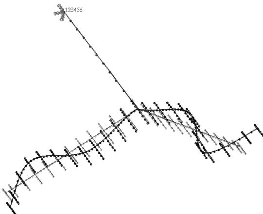
Fig.29 4<sup>th</sup> mode - frequency = 8.2 Hz
