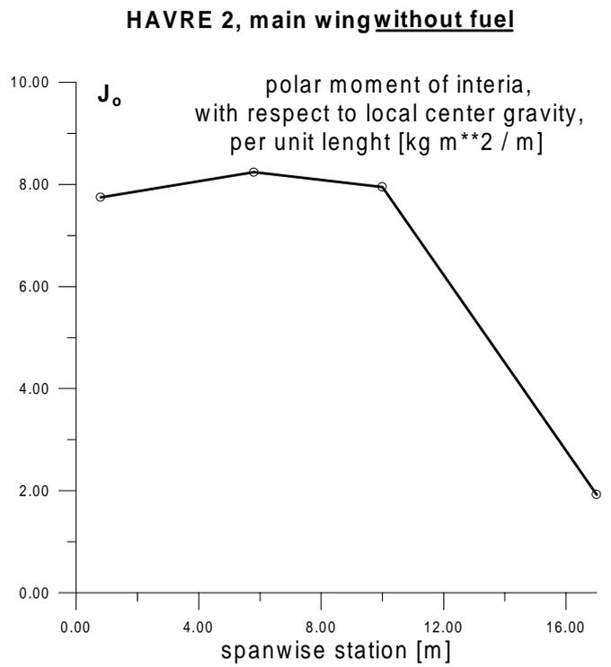
Fig.15 Spanwise distribution of the polar moment of inertia
