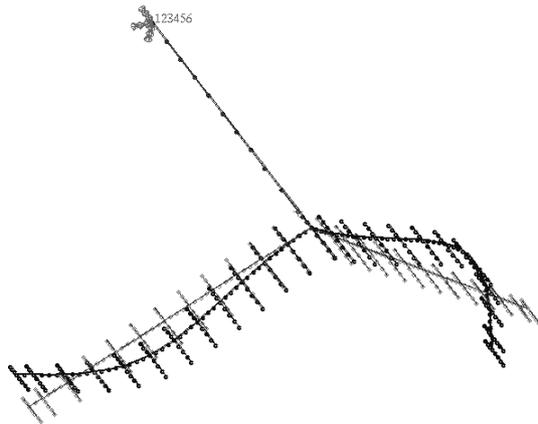
Fig.27 2<sup>nd</sup> mode - frequency = 3.1 Hz
