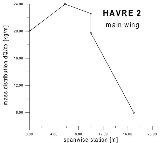
Fig.16 Spanwise mass distribution
