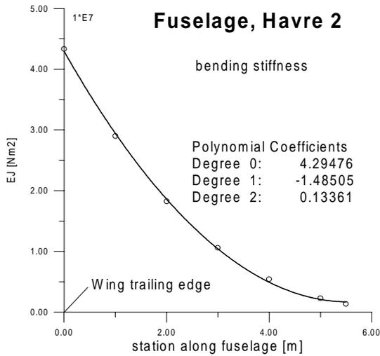
Fig.22 Bending stiffness along fuselage
