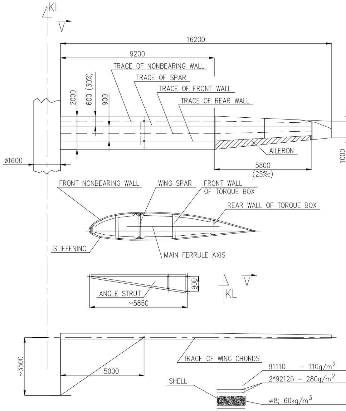
Fig.7 Ribs, spar and torque box
