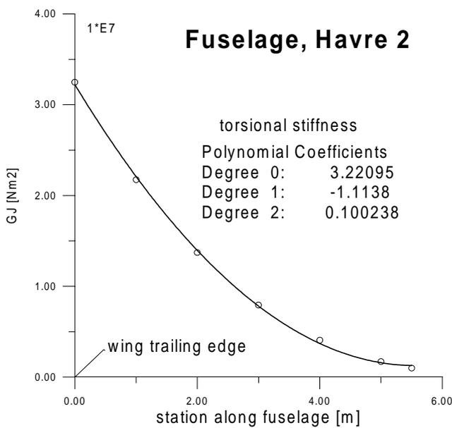
Fig.23 Torsional stiffness along fuselage
