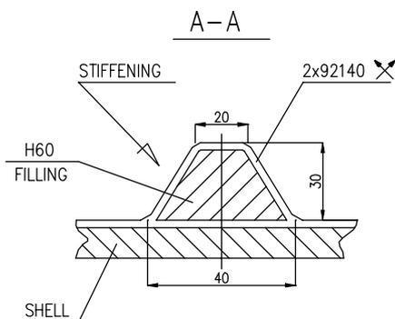
Fig.3 Chordwise stiffening strip section
