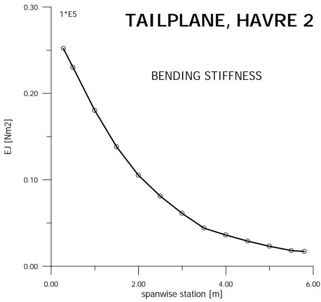
Fig.17 Spanwise distribution of bending stiffness
