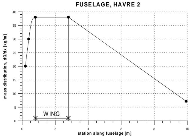
Fig.24 Mass distribution along fuselage
