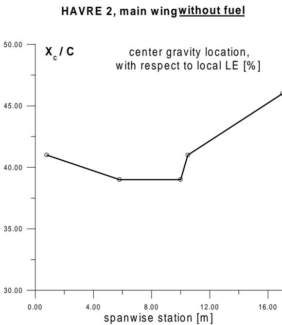
Fig.14 Spanwise distribution of the mass centre location
