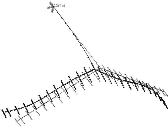
Fig.28 3th mode - frequency = 5.6 Hz
