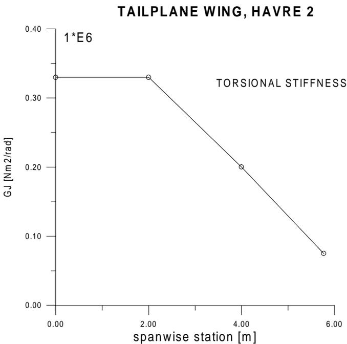
Fig.18 Spanwise distribution of torsional stiffness
