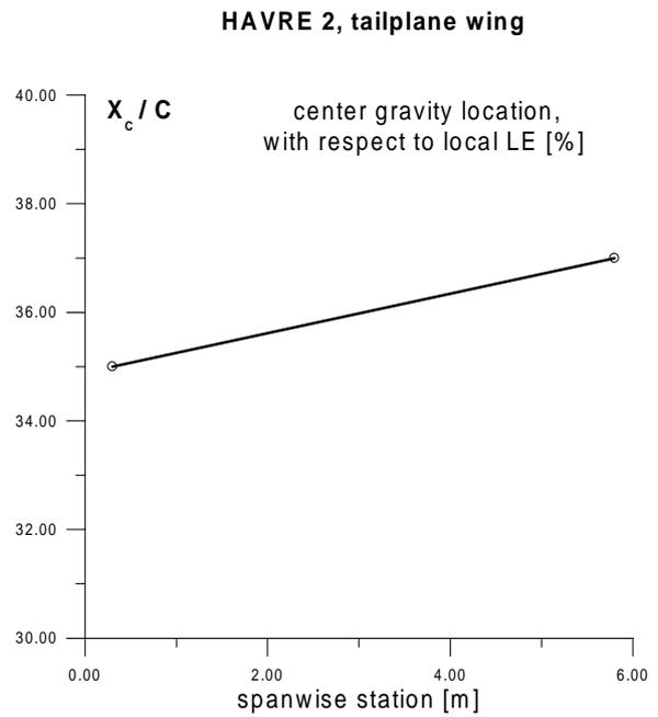
Fig.19 Spanwise distribution of the mass centre location
