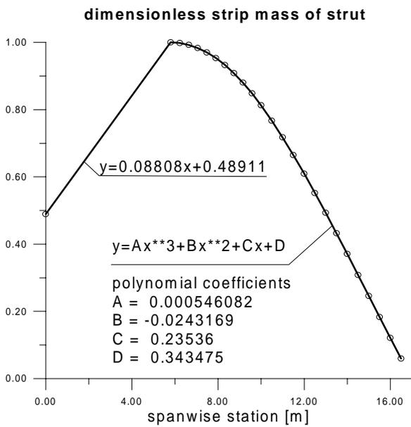
Fig.9 Spanwise mass distribution of the strut
