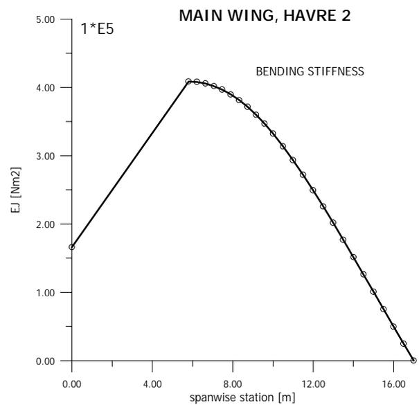
Fig.12 Spanwise distribution of bending stiffness
