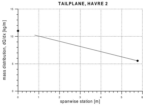
Fig.21 Spanwise mass distribution
