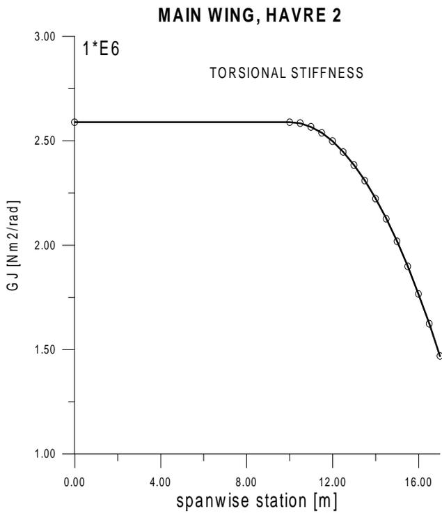
Fig.13 Spanwise distribution of torsional stiffness
