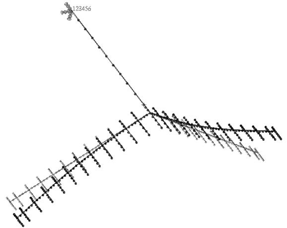
Fig.26 1<sup>st</sup> mode - frequency = 0.8 Hz
