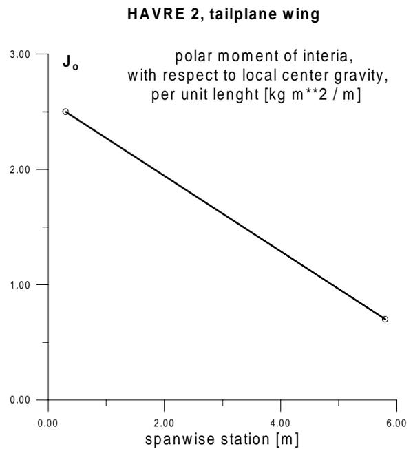
Fig.20 Spanwise distribution of the polar moment of inertia
