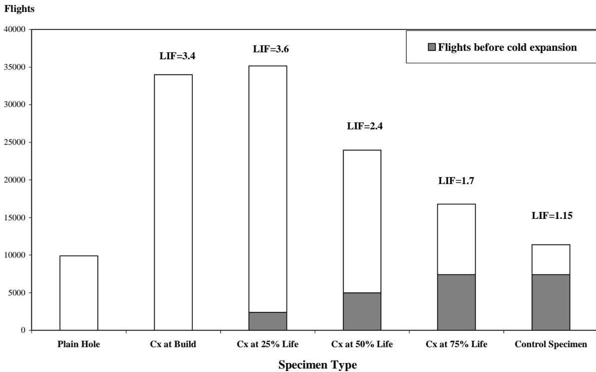
Fig. 2 Test result of part-life cold expanded LLTJ specimens.
