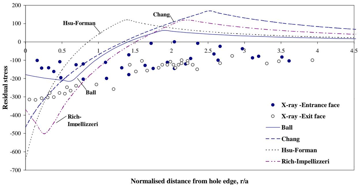
Fig. 4 Residual stress distributions determined by different closed-form models.
