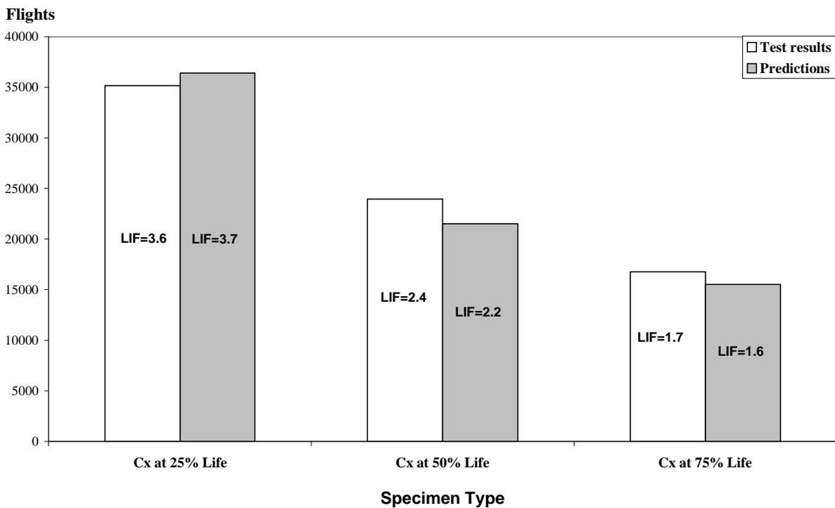
**Fig. 6 Comparison of life improvement factor (LIF) between test and predicted results**
