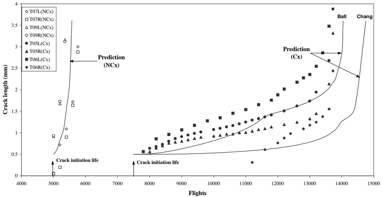
**Fig. 5 Simulation of crack growth histories by AFGROW using two different residual stress models.**
