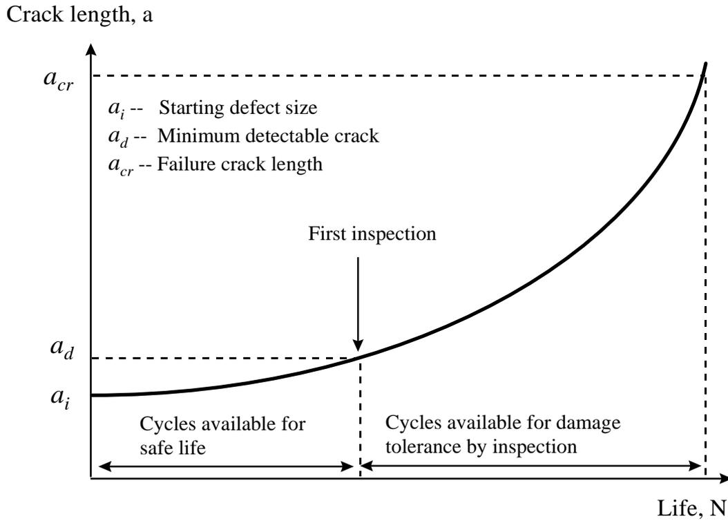
Fig. 3 Prediction of fatigue life by damage tolerance approach.
