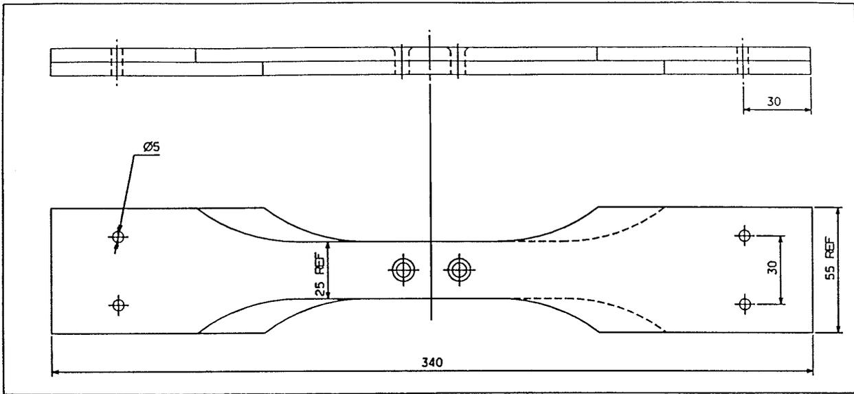
Fig. 1 Low Load Transfer Joint (LLTJ) Specimen.
