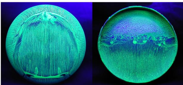
**Figure 3. The surface paint patterns at  $5^\circ$  incidence,  $Re = 2.84 \cdot 10^5$ . (Left) Upper surface. (Right) Cavity surface.**
