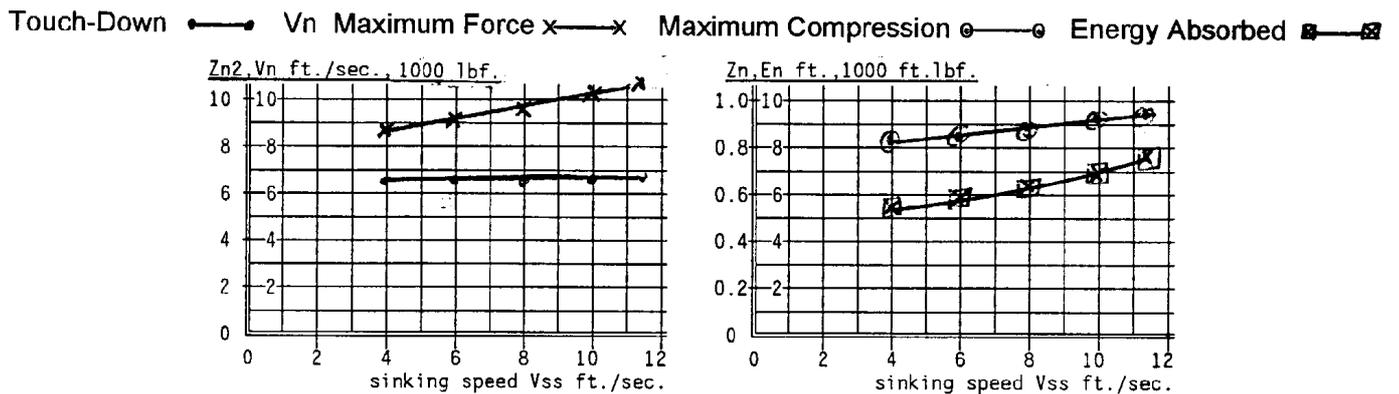
value) is the same at the extreme angles of pitch, with a minimum intermediate value that is considerably less. As noted above, for the main gear this corresponds to a maximum energy absorption peak. On the nose gear, the energy absorbed from the slam down maneuver and the associated maximum vertical forces are greater than for level landing, and the situations due to this operation should not be easily dismissed.
