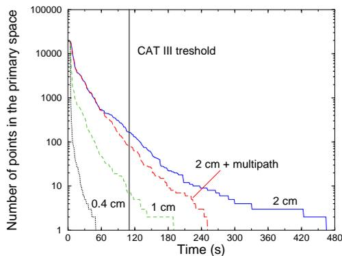
**Fig. 3** Time of convergence of LSAST for different levels of noise.
