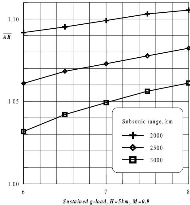
**Fig.3. Relative change of required wing aspect ratio.**
