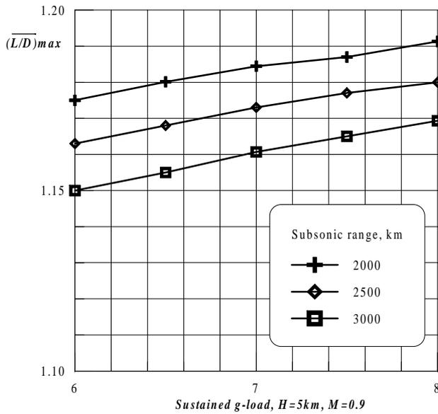
**Fig.2. Relative change of required maximum lift-to-drag ratio**
