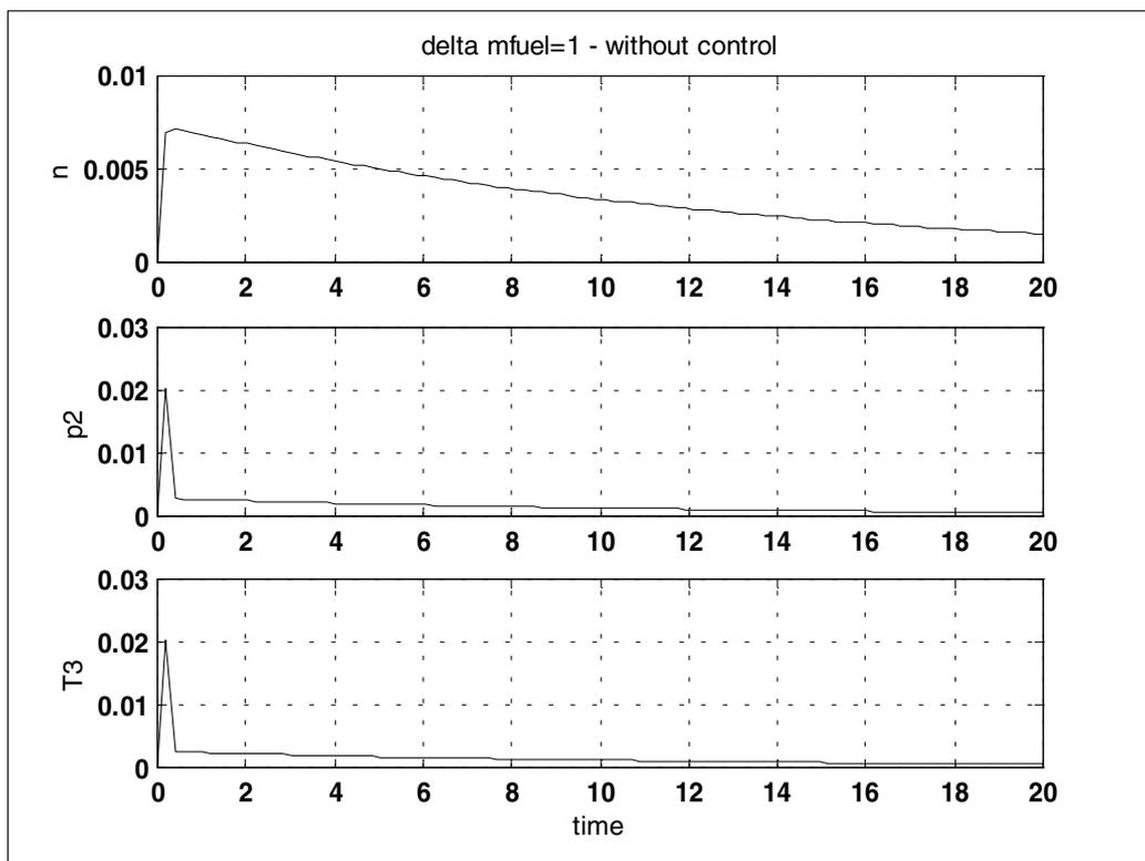
Fig. 1.: Simulation when  $m_{fuel}$  is a Dirac-delta function (without control)
