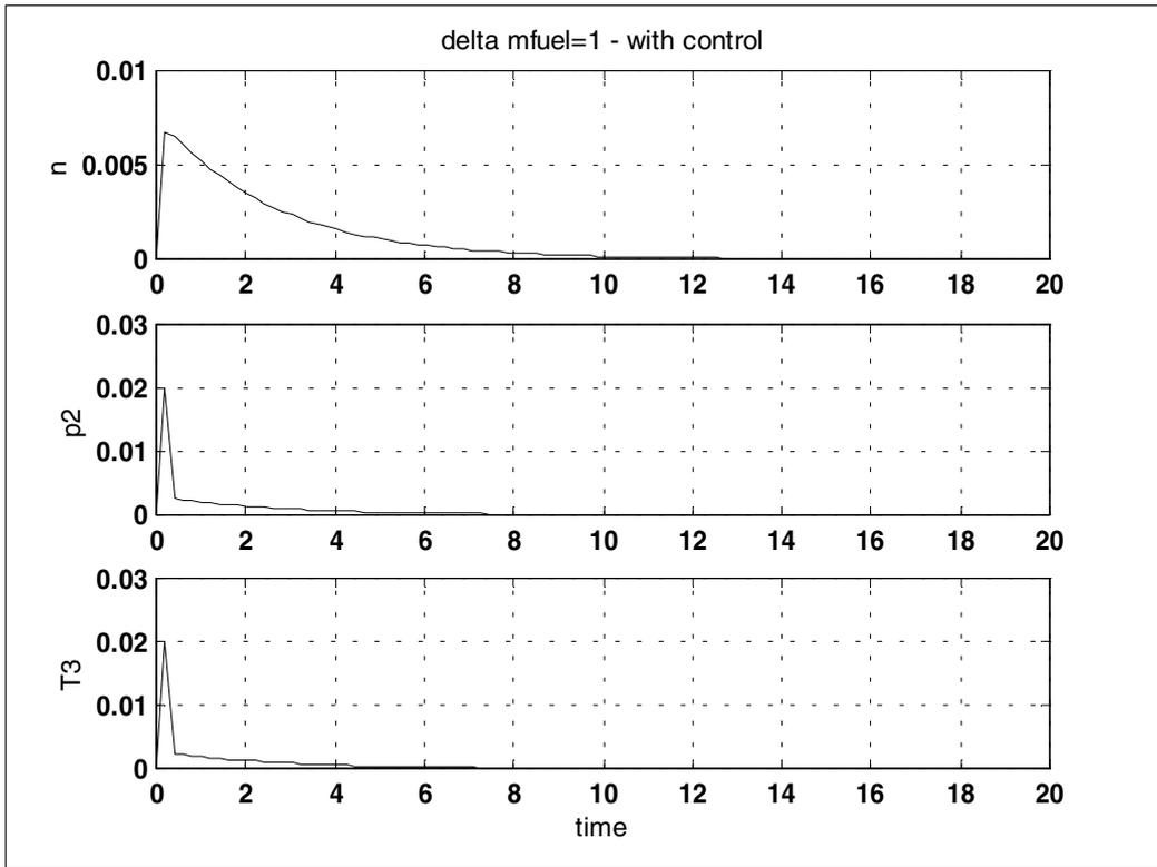
Fig.3.: Simulation when  $m_{fuel}$  is a Dirac-delta function (with LQ control)
