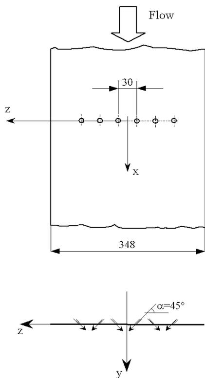
**Fig. 1 Sketch of the flat plate with jet holes configuration and reference system. All dimensions in millimeters.**
