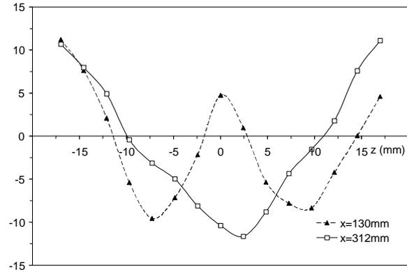
Fig. 4 Percent variation of mean longitudinal velocity for two different sections downstream the injection point and located at a distance  $y+\approx 20$  from the plate.
