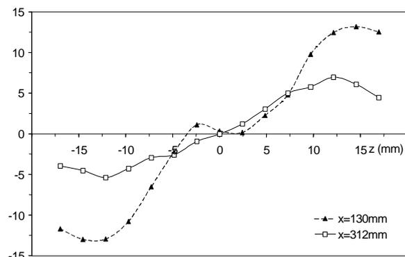
Fig. 5 Mean spanwise velocity distributions for two different sections downstream the injection point and located at a distance  $y+\approx 20$  from the plate.
