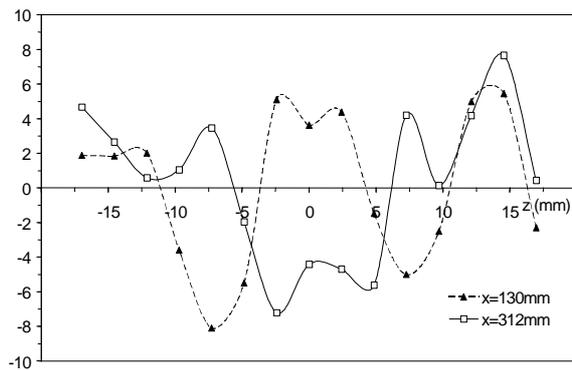
**Fig. 6 Percent variation of streamwise turbulence intensity for two different sections downstream the injection point and located at a distance  $y+\approx 20$  from the plate.**
