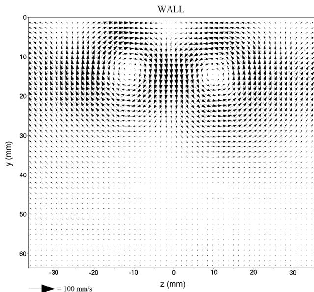
**Fig. 2 Mean vectorial velocity flow field in the (y,z) plane at x=130mm.**
