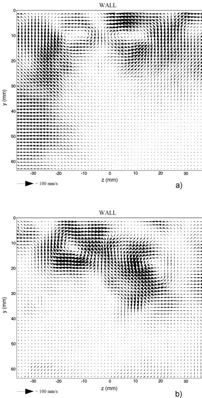
Fig. 3 Instantaneous vectorial velocity flow fields in the (y,z) plane at x=130mm.
