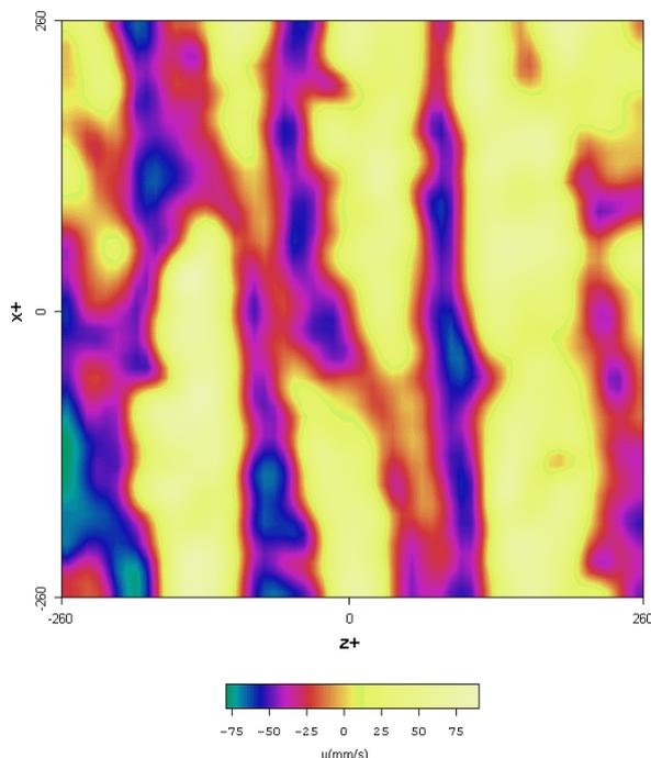
**Fig. 7 Grey level map of streamwise fluctuating velocity component in the  $(y,z)$  plane centered at  $x=312\text{mm}$ . Jets off;  $y+\approx 20$ .**
