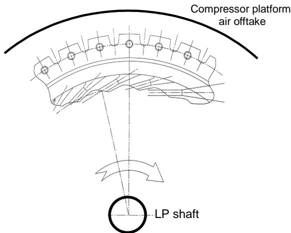
**Fig. 5: Schematic view of tubeless vortex reducer**
