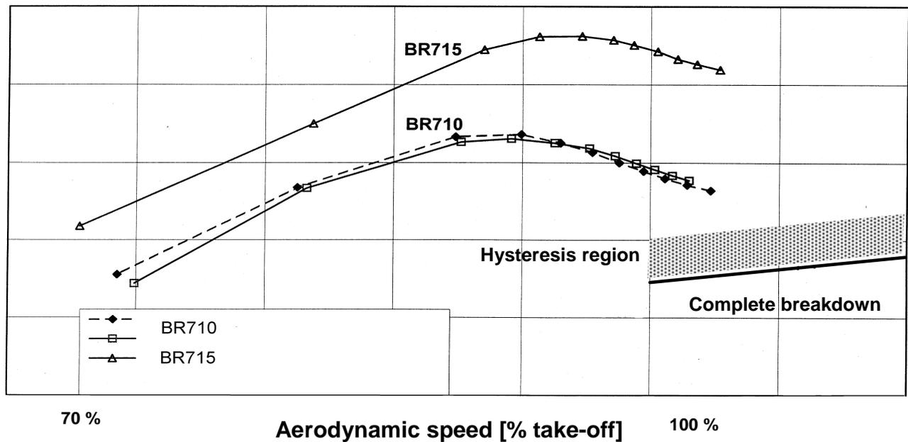
Fig. 10: Vortex reducer available pressure ratio as function of aerodynamic speed  $NH/\sqrt{T}$
