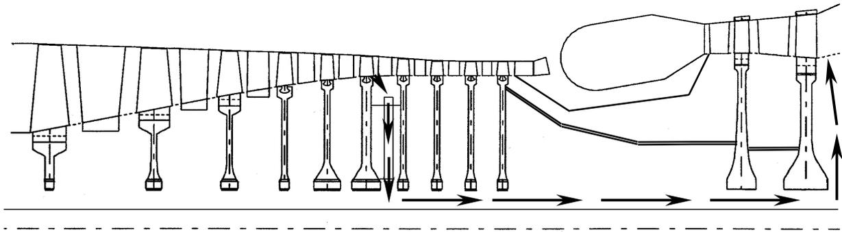
Figure 1: Internal bleed air system scheme
