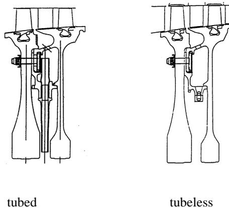
**Fig. 2: Comparison of tubed vs. tubeless vortex reducers**
