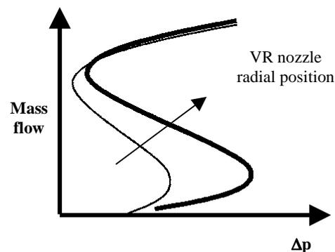
**Fig. 8: Tubeless vortex reducer flow function:
