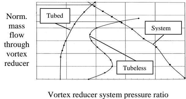
**Fig. 4: Vortex reducer system flow characteristics**
