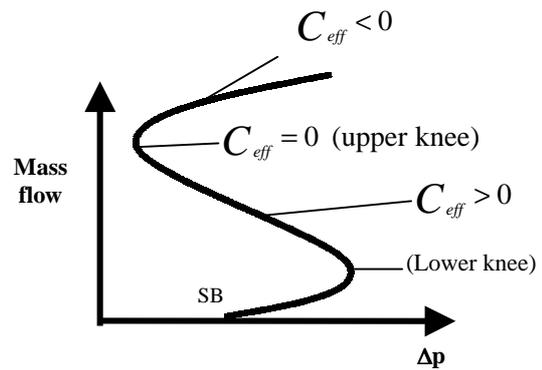
**Fig. 6: Flow regimes of tubeless vortex reducer**
