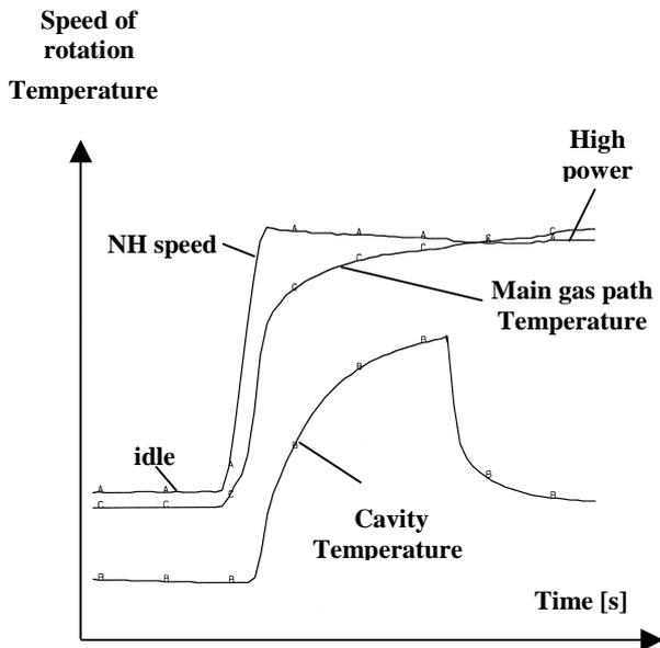
Fig. 11: Turbine cavity and main gas path temperature at slam accel to vicinity of breakdown line
