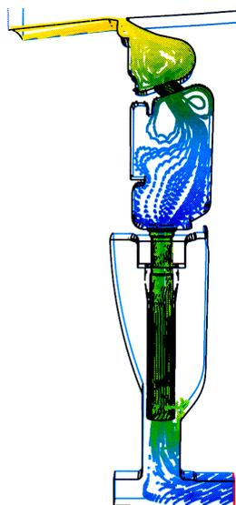
Fig. 12: 3-D CFD solution of tubed vortex reducer (streamlines colored by velocity)
