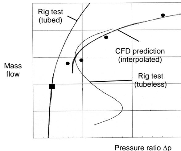
Fig. 13: Validation of CFD calculation with vortex reducer rig test results
