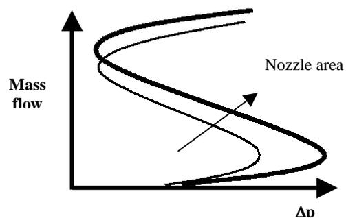
**Fig. 7: Tubeless vortex reducer flow function: Effect of nozzle area**
