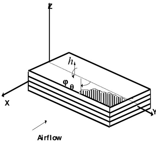
Fig. 1. Coordinate system and notation for a composite wing idealised as a beam element.
