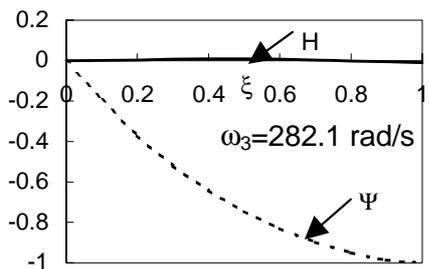
Fig. 2 Natural frequencies and mode shapes of a composite wing with  $[-8^0]_{14}$  layup
