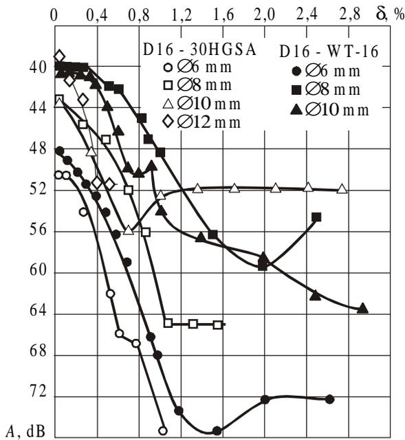
**FIGURE 2. Dependence of amplitude of an echo of a shear wave to value of relative clearance**
