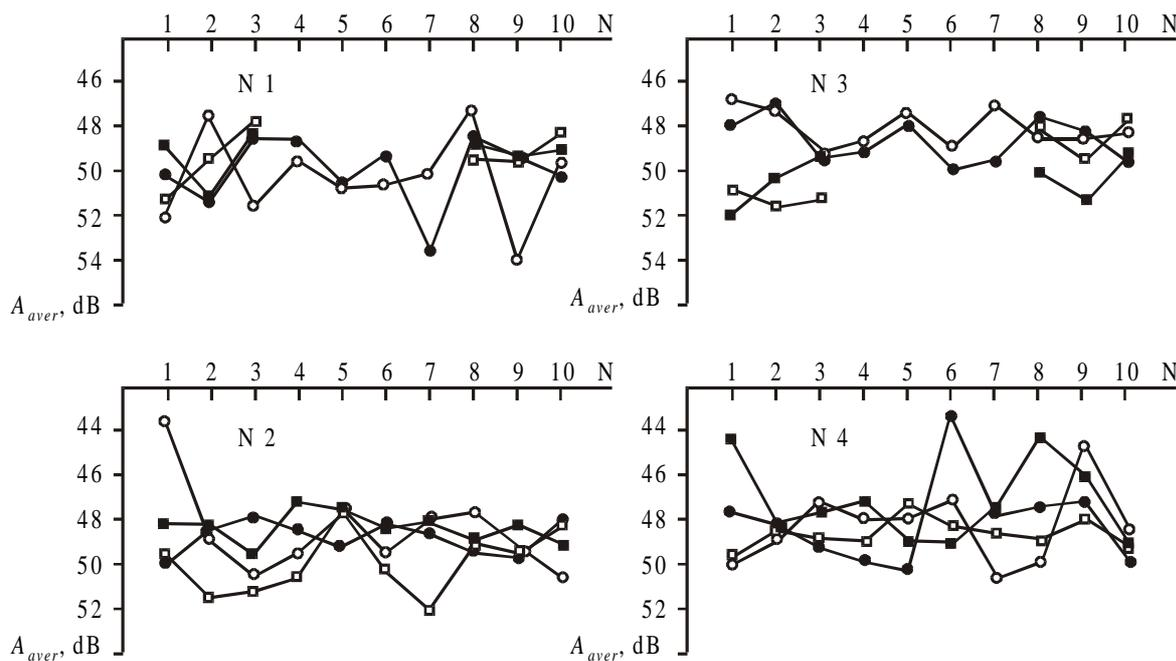
FIGURE 9. The charts of distribution of echo-signal amplitude average values in each raw for four hatches
