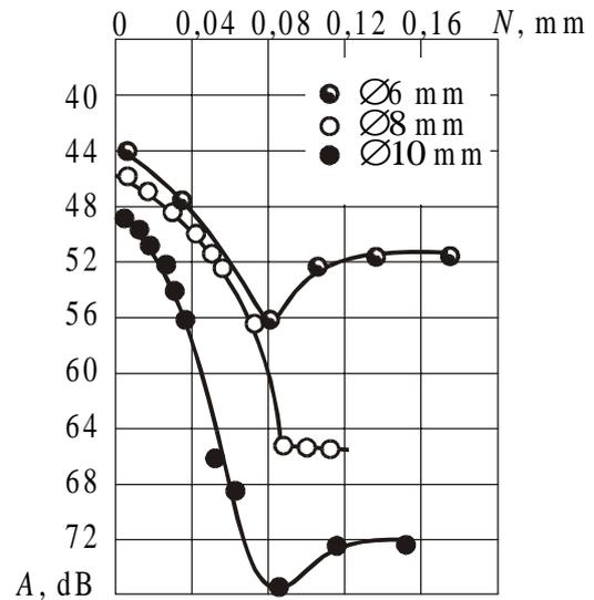
**FIGURE 3. Dependence of amplitude of an echo of a shear wave to value of absolute clearance for a contact D16-30HGSA**
