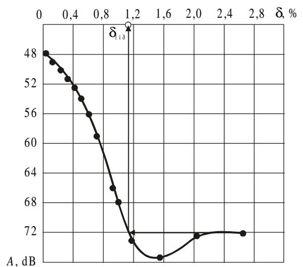
**FIGURE 4. The scheme of definition of the upper limit of range of a unambiguous estimation of interference on amplitude characteristic (D16-HGSA Ø6 mm)**
