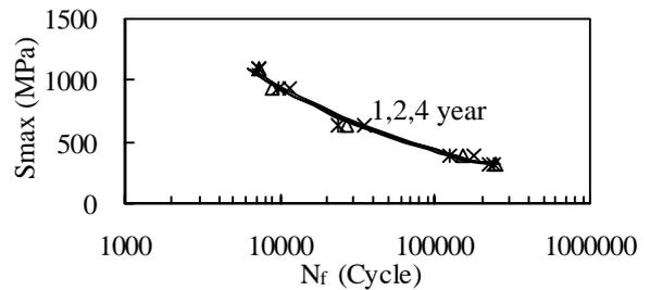
Fig.3b: S-N curves for 30CrMnSiNi2A plain specimen
