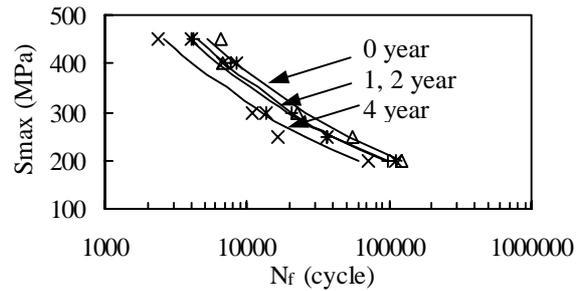
Fig.3a: S-N curve for LC4CS plain specimen
