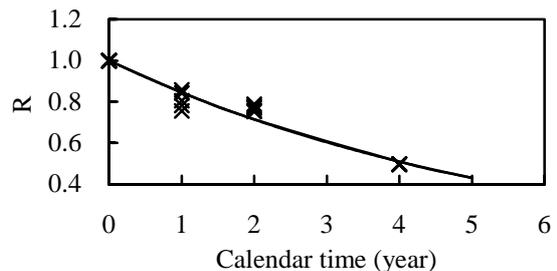
Fig.4b: R-y fitting curve for LC4CS plain specimen
