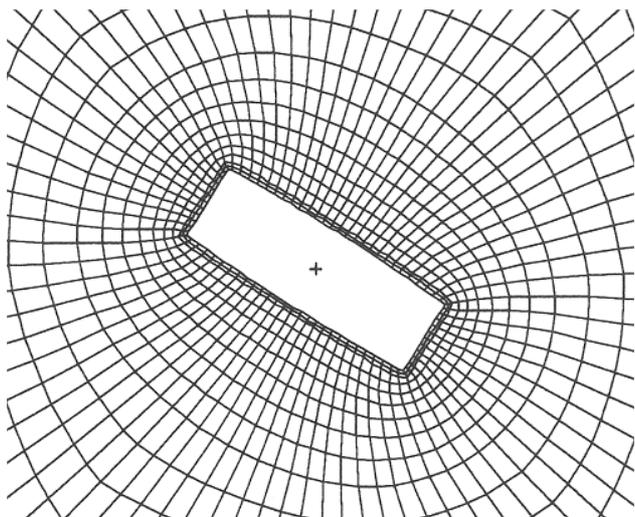
Figure 10 Optimum cut-out under 1:1 shear/compression loading for an isotropic plate
