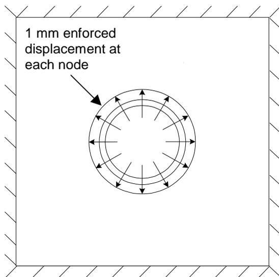
Figure 3 Auxiliary model for shape optimisation showing loads and boundary conditions
