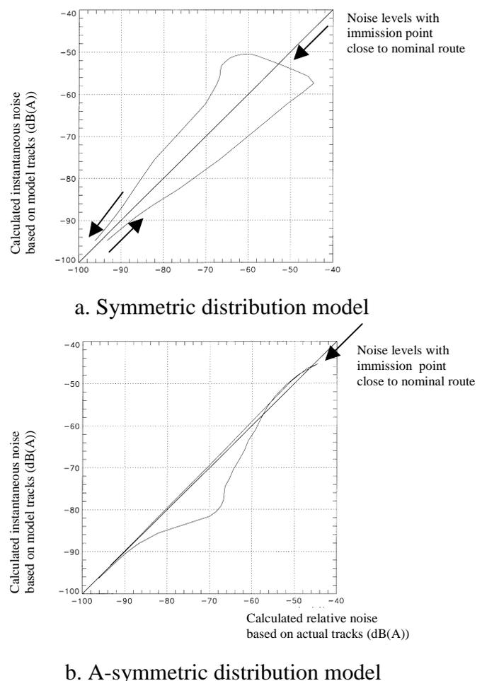
**Figure 4** Relative noise level for modelled distribution versus relative noise level for actual dispersion (dB(A)).
