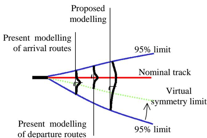
Figure 0 Modelling of lateral track dispersion
