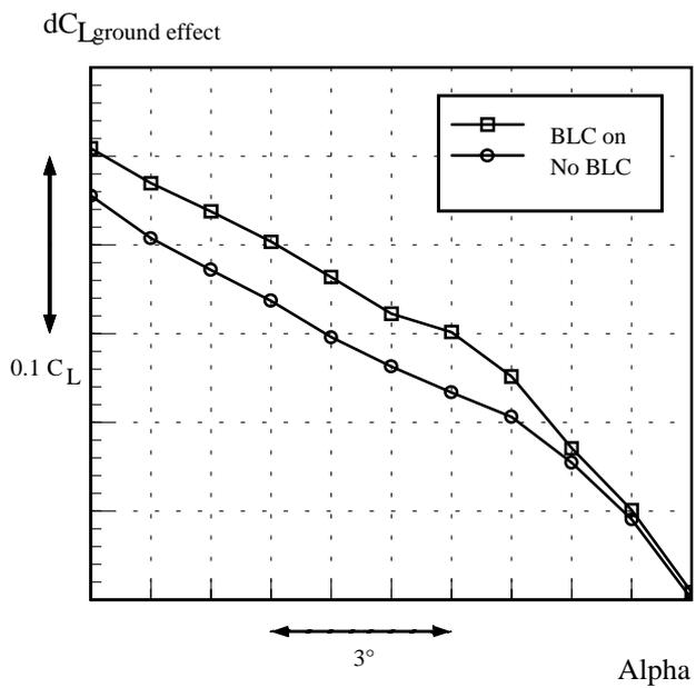
**Figure 11** Influence of boundary layer control on ground effect on A3XX, aircraft-on-ground
