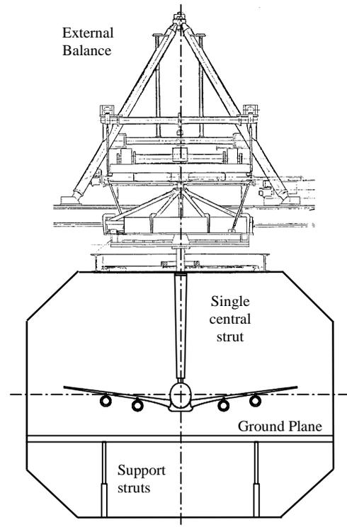
Figure 2. Ground effect testing arrangement
