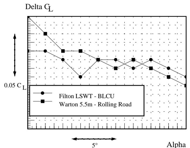
**Figure 8 Comparison of  $C_L$  increments due to the rolling road or BLCU**
