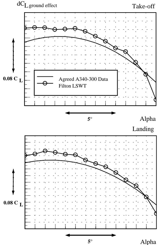
**Figure 9 Ground effect comparisons for the A340-300**
