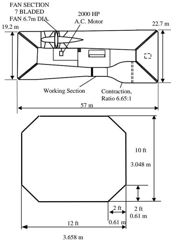
Figure 1. The Filton Low Speed Wind Tunnel circuit plan and working section geometry
