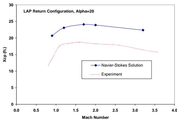
Fig 8 LAP X<sub>cp</sub> vs M, α=20°
