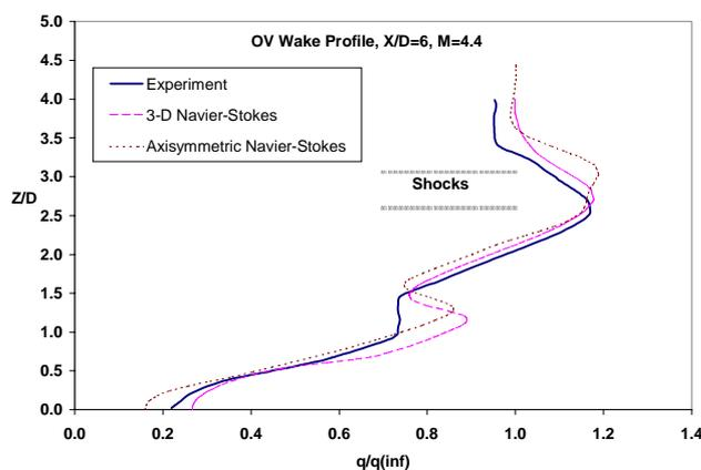
Fig 11 OV Wake Dynamic Pressure Profile, M=4.4, X/D=6
