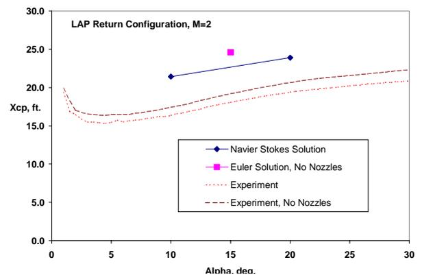
Fig 6 LAP  $X_{cp}$  vs Alpha, M=2
