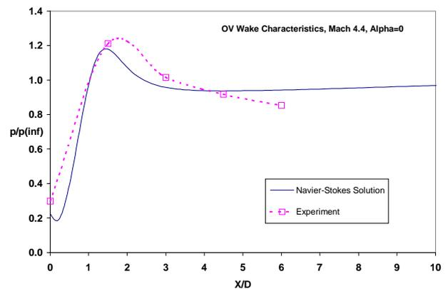
Fig 10 OV Wake Pressure Ratio
