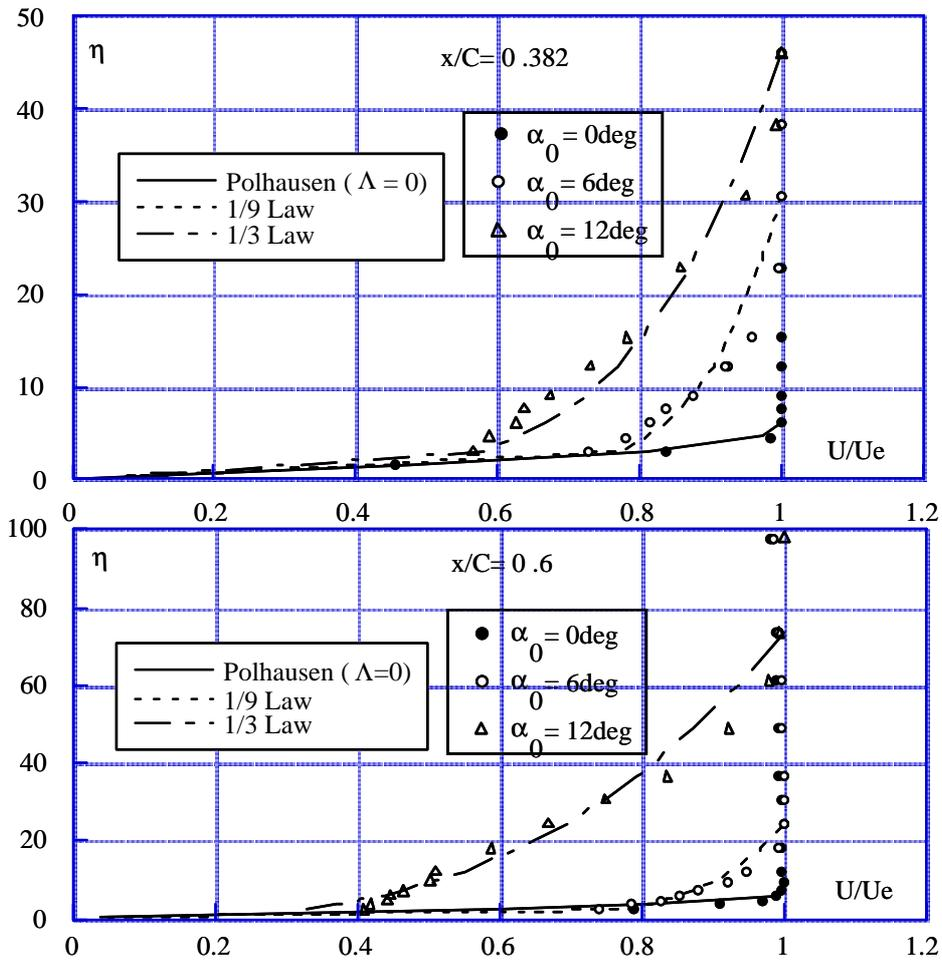
Fig. 4 U-velocity distribution, Steady flow as a function of  $\alpha_0$ .
