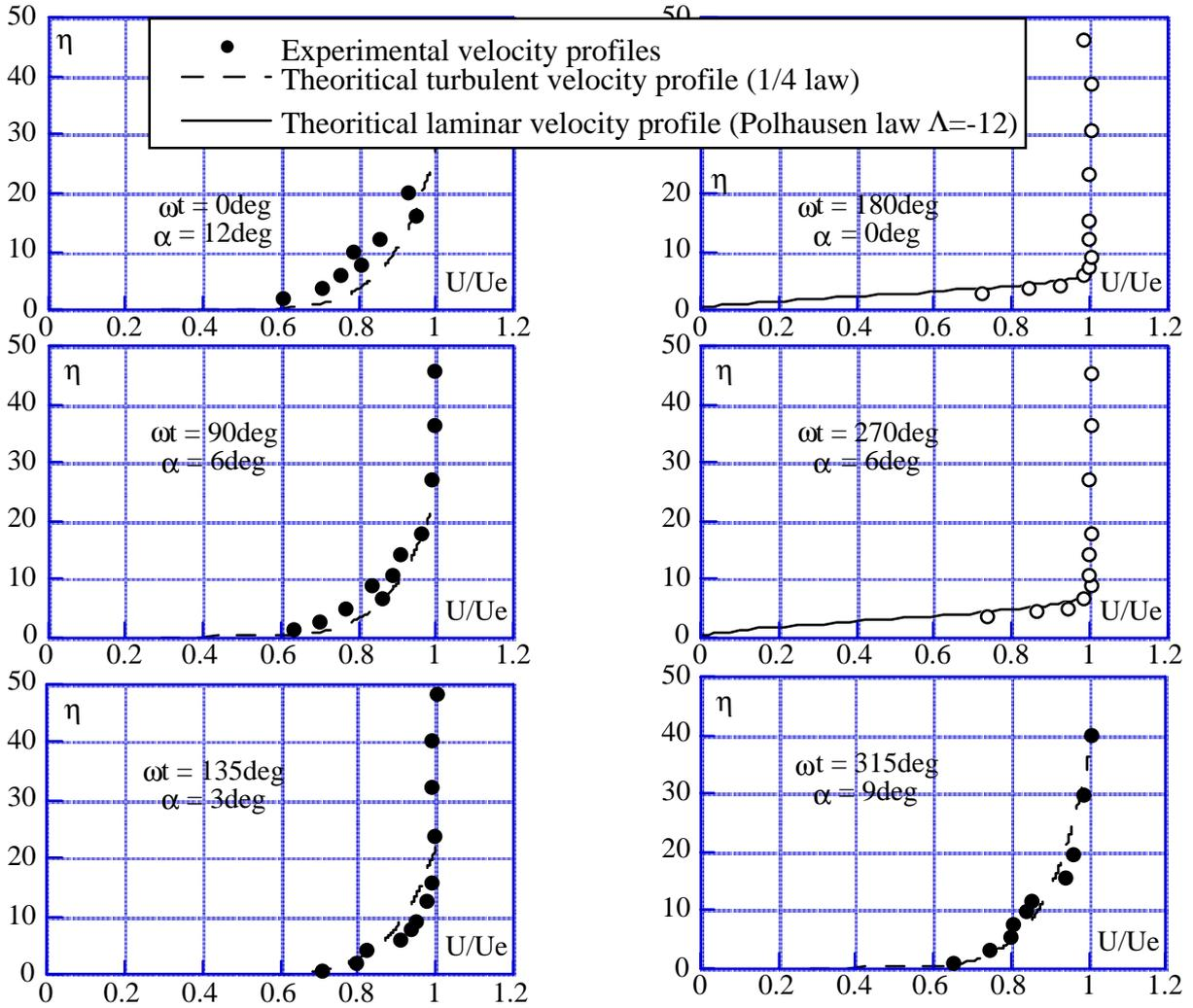
Fig. 8  $U/U_e = U/U_e(\eta)$  in translation/pitch motion.
