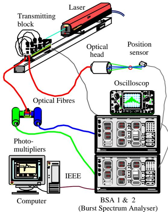
Fig. 3 ELDV data acquisition system.
