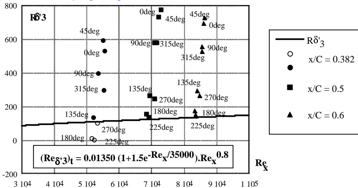
Fig. 7 Transition criterion in pitching motion.
