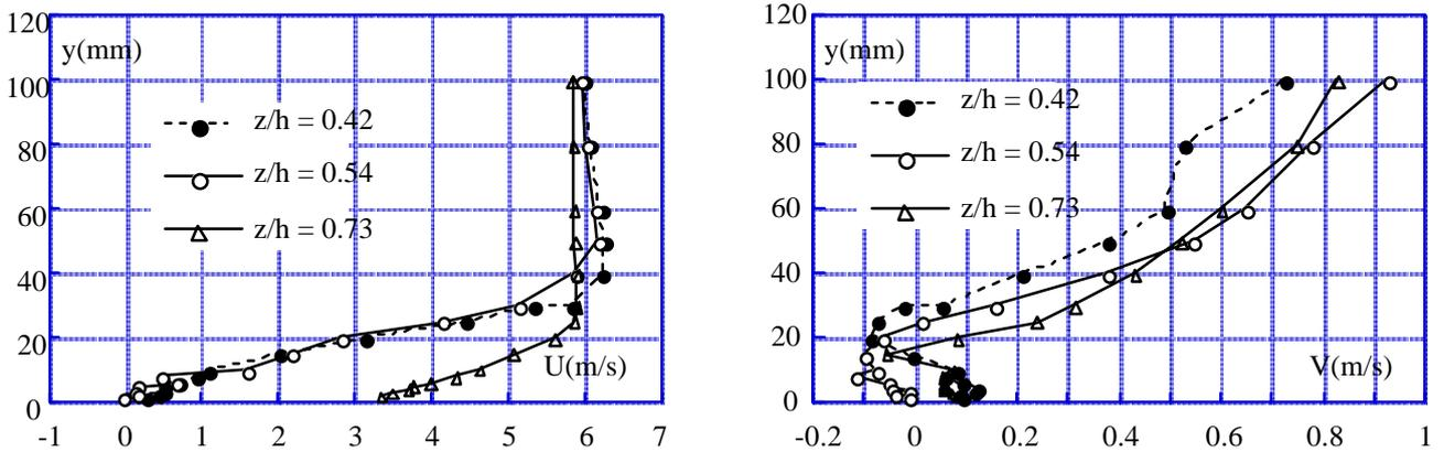
Fig. 5 U-velocity distribution, Steady flow as a function of  $z/h$ .
