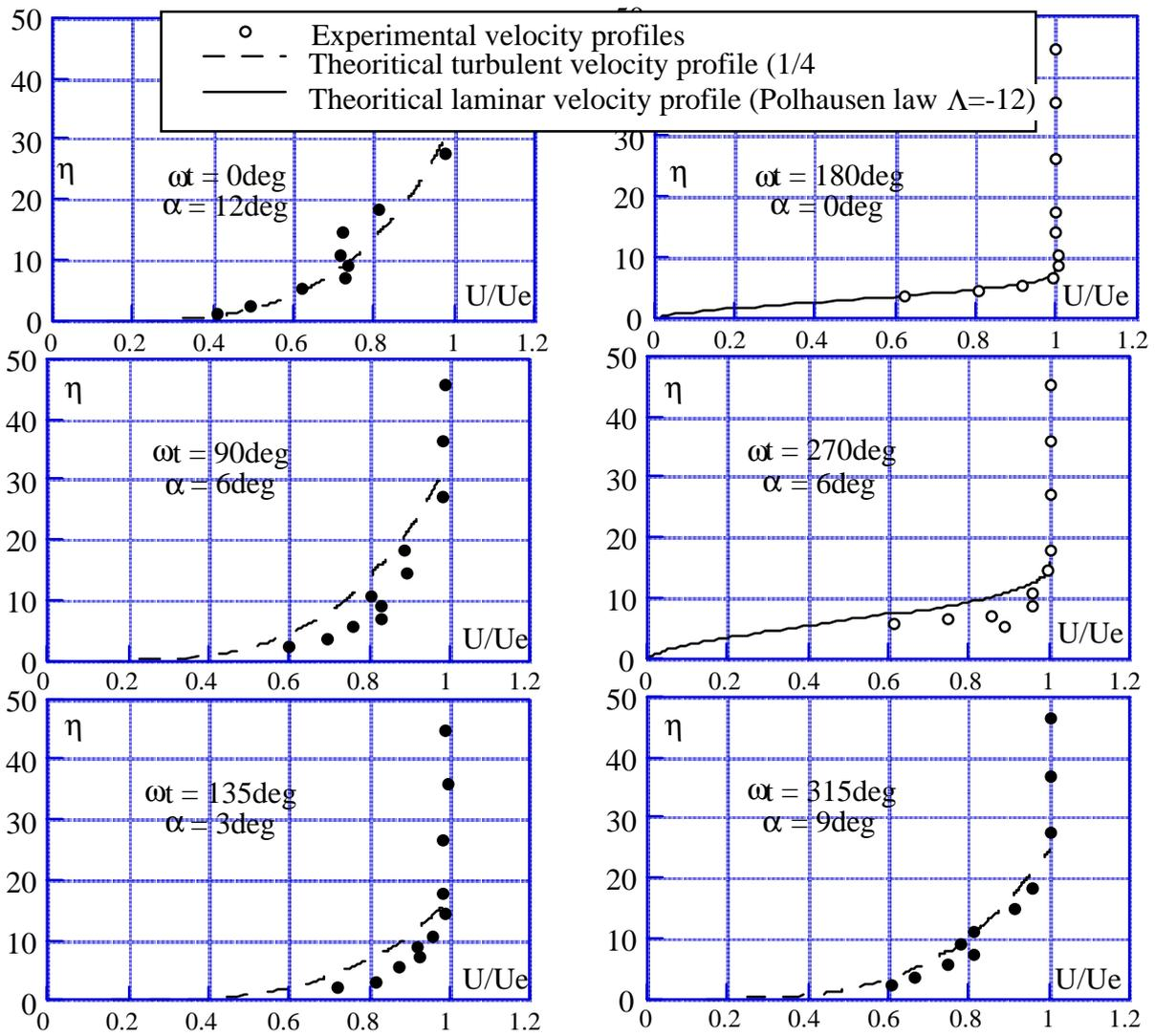
Fig. 6  $U/U_e = U/U_e(\eta)$  in pitching motion.
