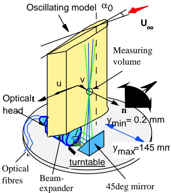
Fig. 2 Embedded optical head linked with the oscillating model.
