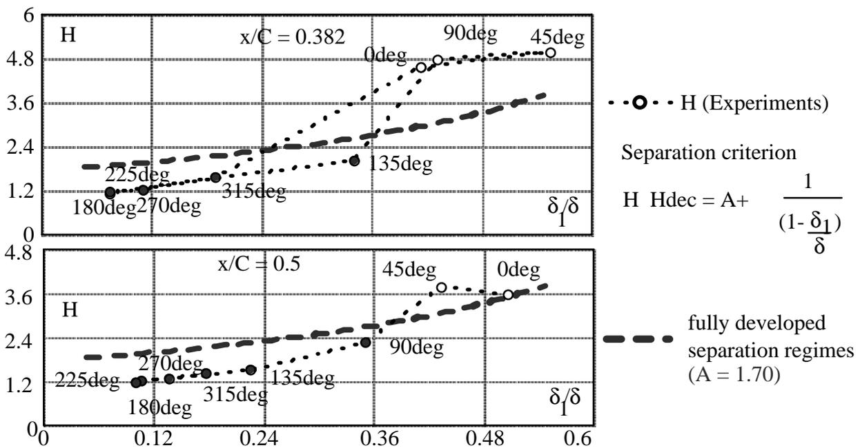
Fig. 11 Separation criterion in pitch- $\alpha=12\text{deg}$ .
