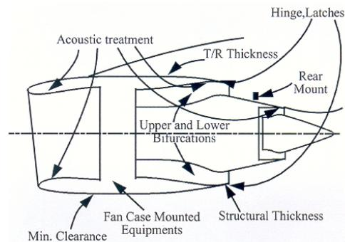
Figure 6: Nacelle hardware requirements
