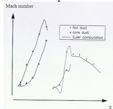
**Figure 29: CFD and experimental results in fan duct and core duct**
