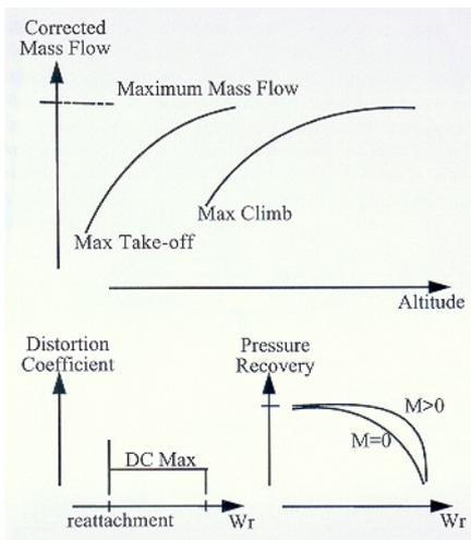
Figure 4: Engine requirements
