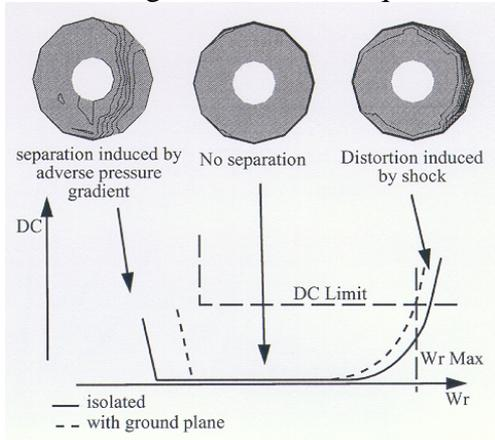
**Figure 25: Distortion Coefficient (DC) versus engine mass flow (Wr) in cross wind conditions**
