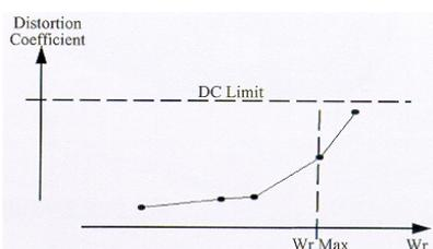
Figure 22: Inlet / Engine compatibility
