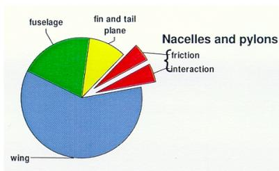
**Figure 1: Typical airframe drag breakdown**
