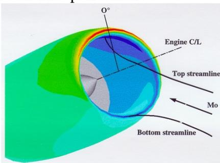
**Figure 26: Local Mach number, High incidence, low mass flow**
