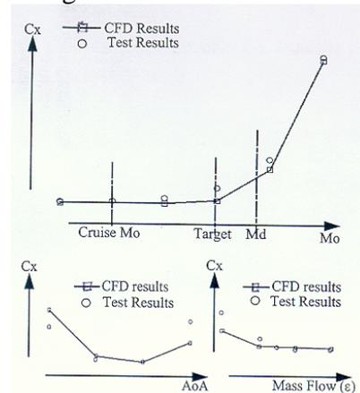
Figure 18: S1 isolated inlet drag results
