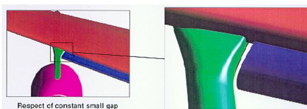
**Figure 2: Gap between pylon and deployed slat**
