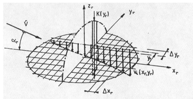
Airflow over the rotor disk
