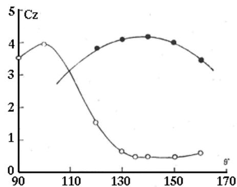
Fig. 5. Comparison of tests in tunnel and under rotor;  $C_\mu=0.4$ ,  $h=1.4\text{mm}$ ,  $\circ$  test in tunnel;  $\bullet$  test under rotor.
