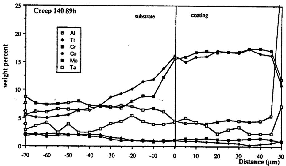
Figure 1 : diffusion profiles for 89 hours at 140 MPa and 1323 K .
