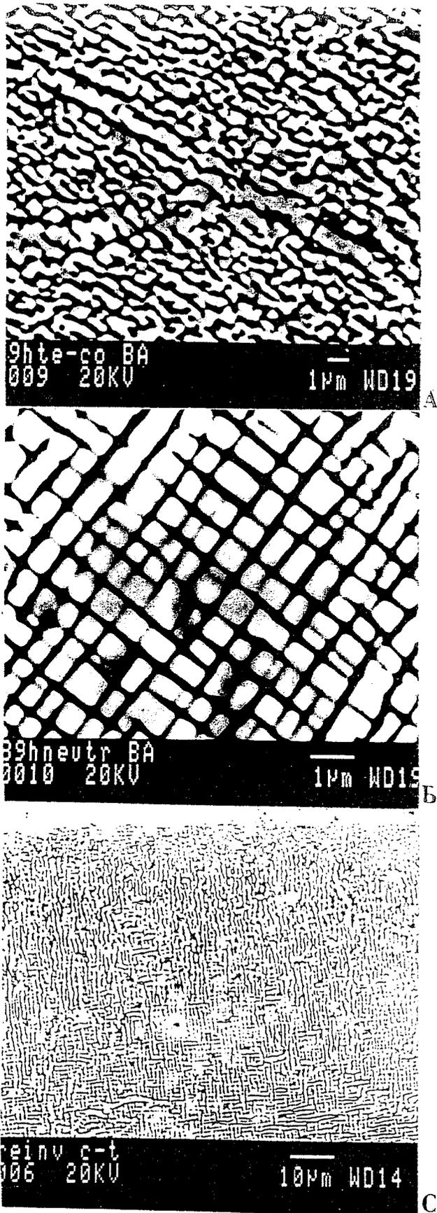
Figure 7: Microstructure after 89 hours of four point bending fatigue test.
