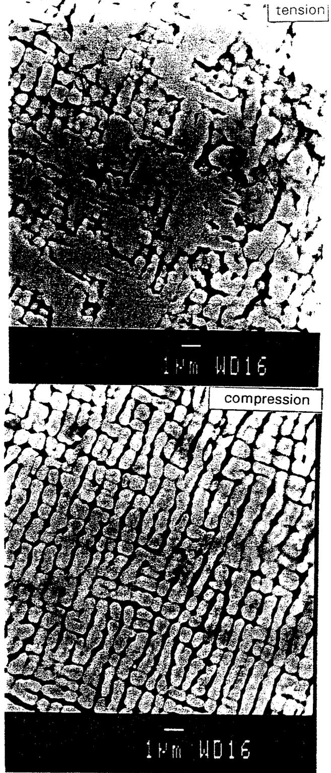
Figure 4: Microstructure after 8 hours of four point bending fatigue test.
