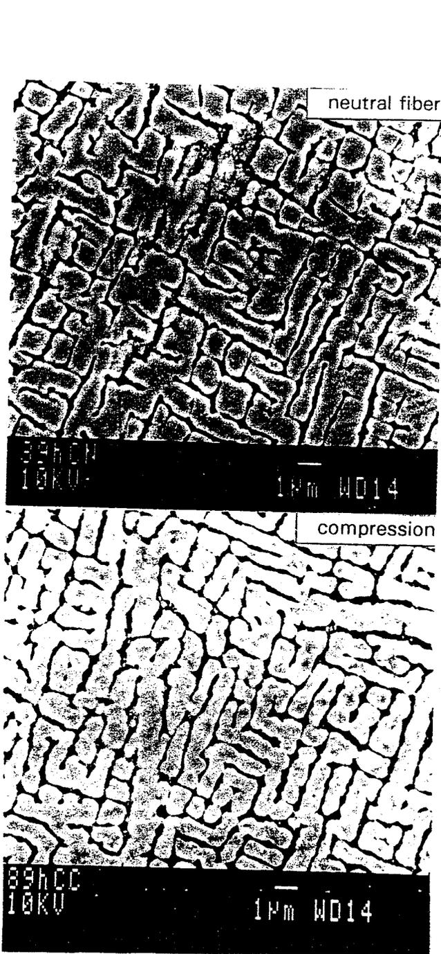
Figure 3: Microstructure after 89 hours of four point bending fatigue test.
