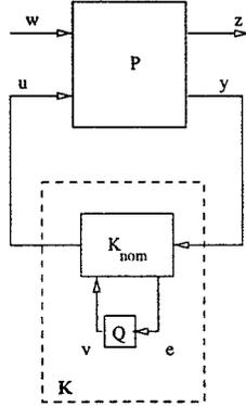
Fig. 2. Q-parameterization as a modification of a nominal controller.
