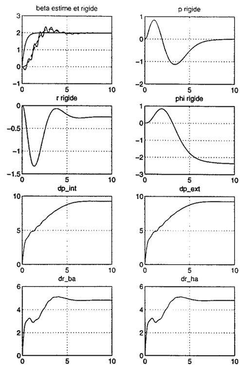
Fig. 8. Step response on the sideslip angle -  $\gamma = 1$ , Q static.
