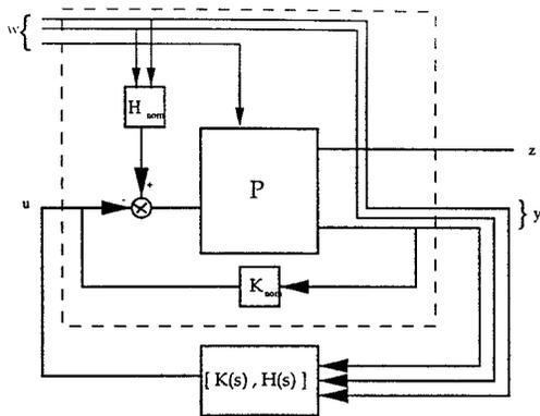
Fig. 4. Augmented Plant with initial feedback  $K_{nom}$  and feedforward  $H_{nom}$
