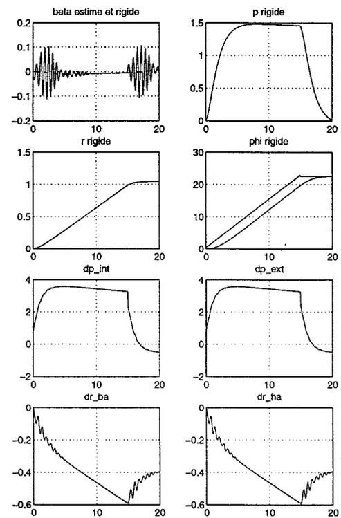
Fig. 9. Step response on the roll rate output -  $\gamma = 1$ , Q static.
