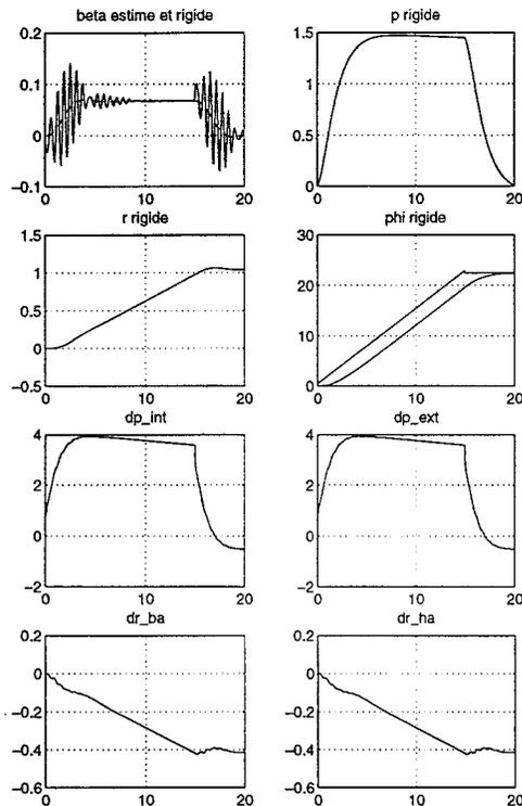
Fig. 7. Step response on the roll rate output - Nominal controller.
