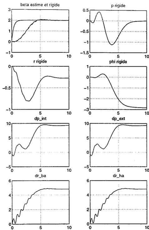
Fig. 10. Step response on the sideslip angle -  $\gamma = 1$ , Q dynamic.
