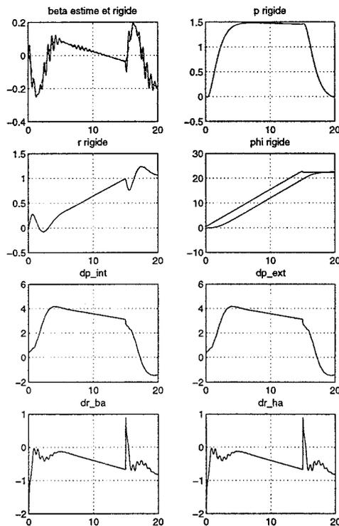
Fig. 11. Step response on the roll rate output -  $\gamma = 1$ , Q dynamic.
