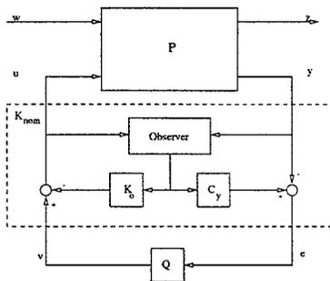
Fig. 3. Q-parametrization in the case of an estimated state feedback nominal controller.  $K_o$  is a state feedback gain and  $y = C_y x$  where  $x$  is the plant state.
