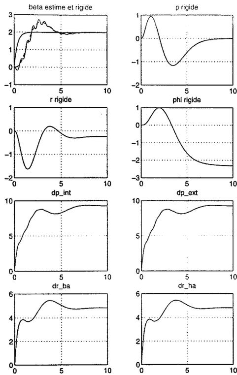
Fig. 6. Step response on the sideslip angle - Nominal controller.
